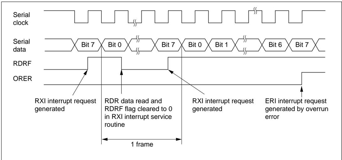
**Figure 14-19 Example of SCI Operation in Reception**
