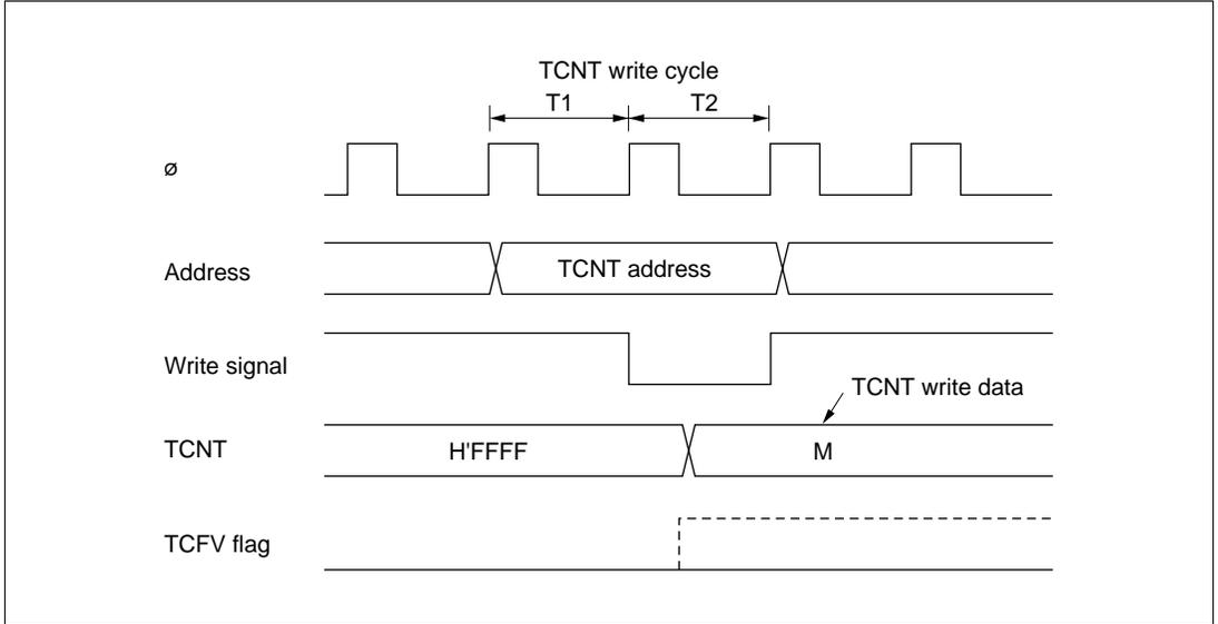
**Figure 10-57 Contention between TCNT Write and Overflow**
