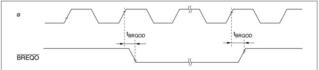
Figure 22-17 External Bus Request Output Timing
