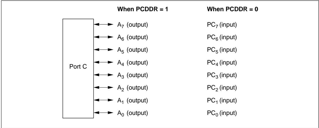
**Figure 9-17 Port C Pin Functions (Mode 6)**
