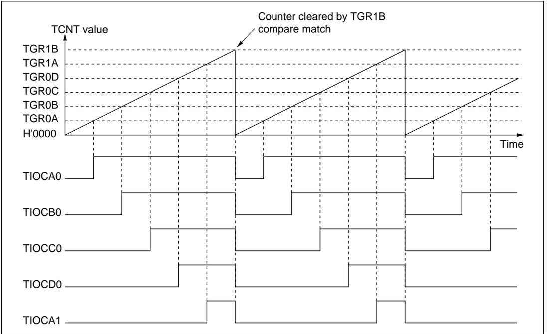
**Figure 10-26 Example of PWM Mode Operation (2)**
