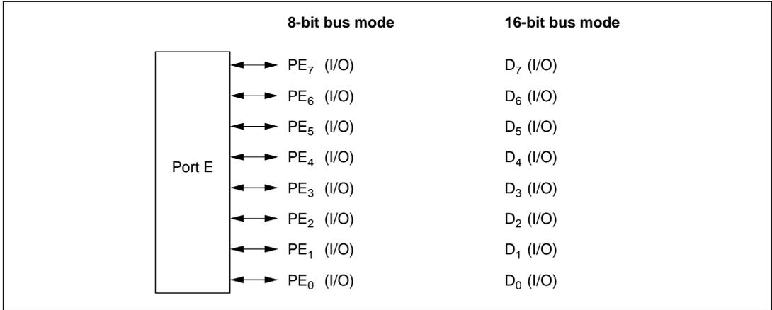
**Figure 9-23 Port E Pin Functions (Modes 4, 5, and 6)**
