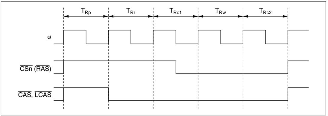
**Figure 6-26 CBR Refresh Timing (When RCW = 1, RLW1 = 0, RLW0 = 1)**
