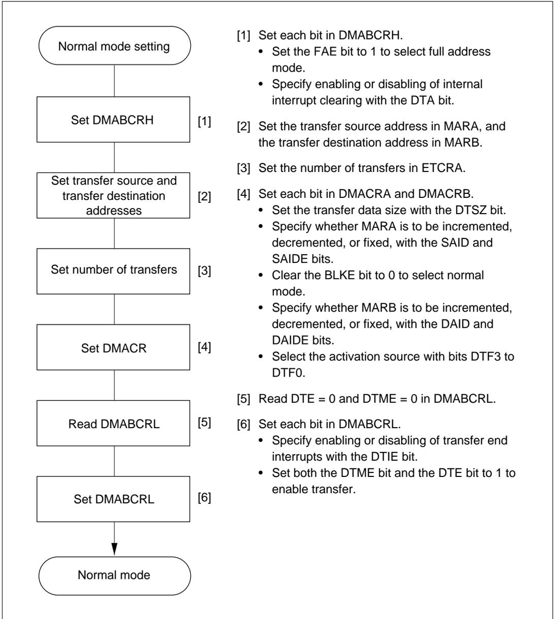
**Figure 7-12 Example of Normal Mode Setting Procedure**
