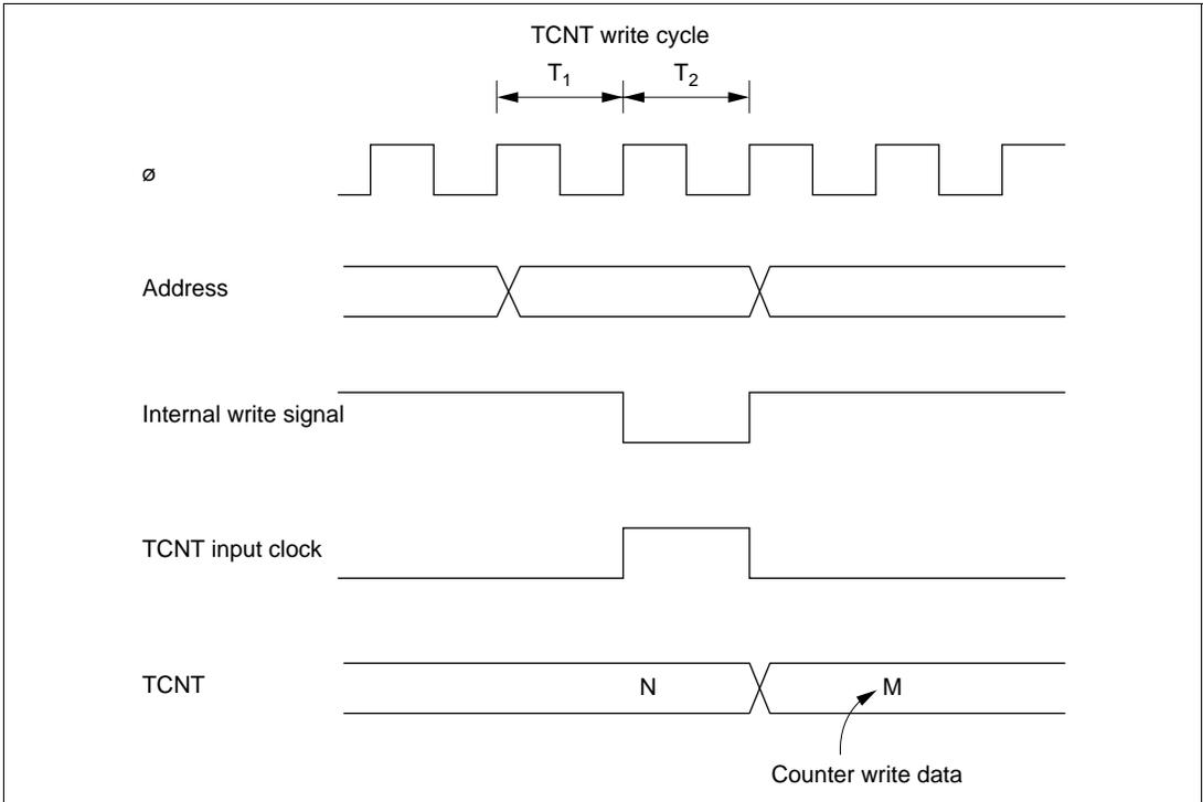
Figure 13-8 Contention between TCNT Write and Increment
