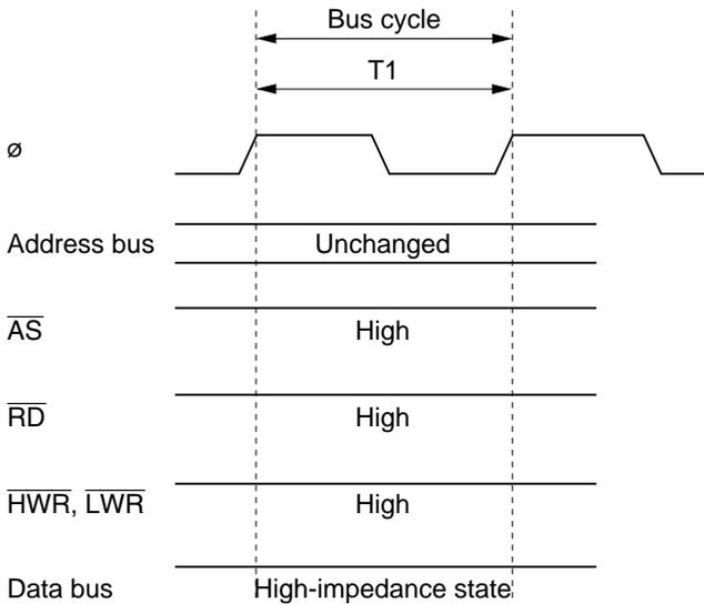
**Figure 2-15 Pin States during On-Chip Memory Access**
