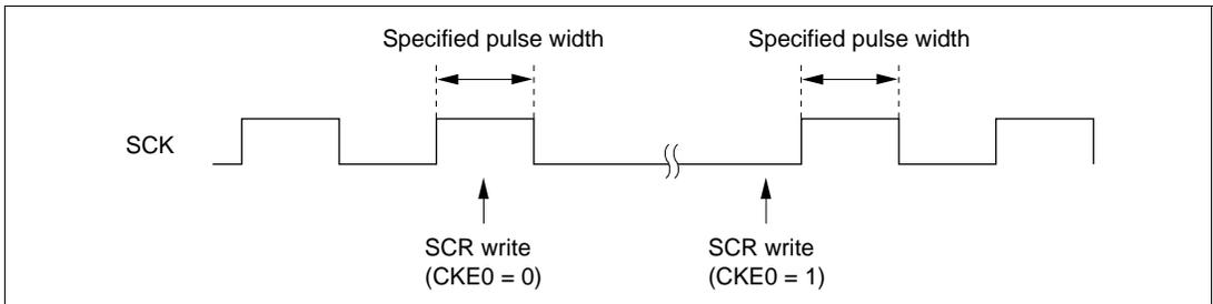
**Figure 15-8 Timing for Fixing Clock Output Level**
