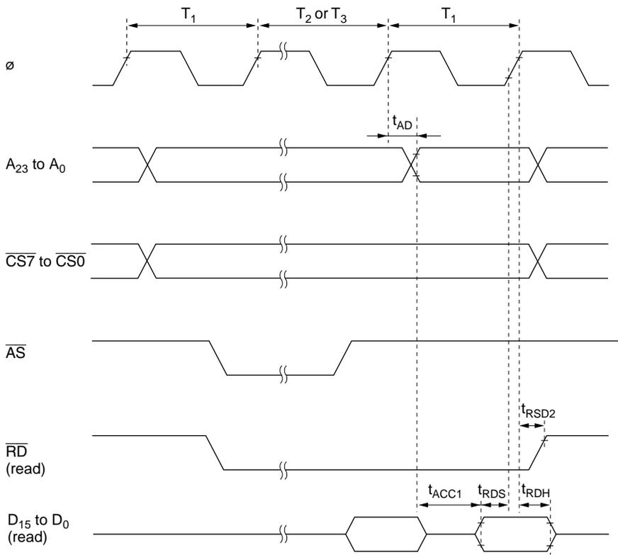
**Figure 22-15 Burst ROM Access Timing (One-State Access)**
