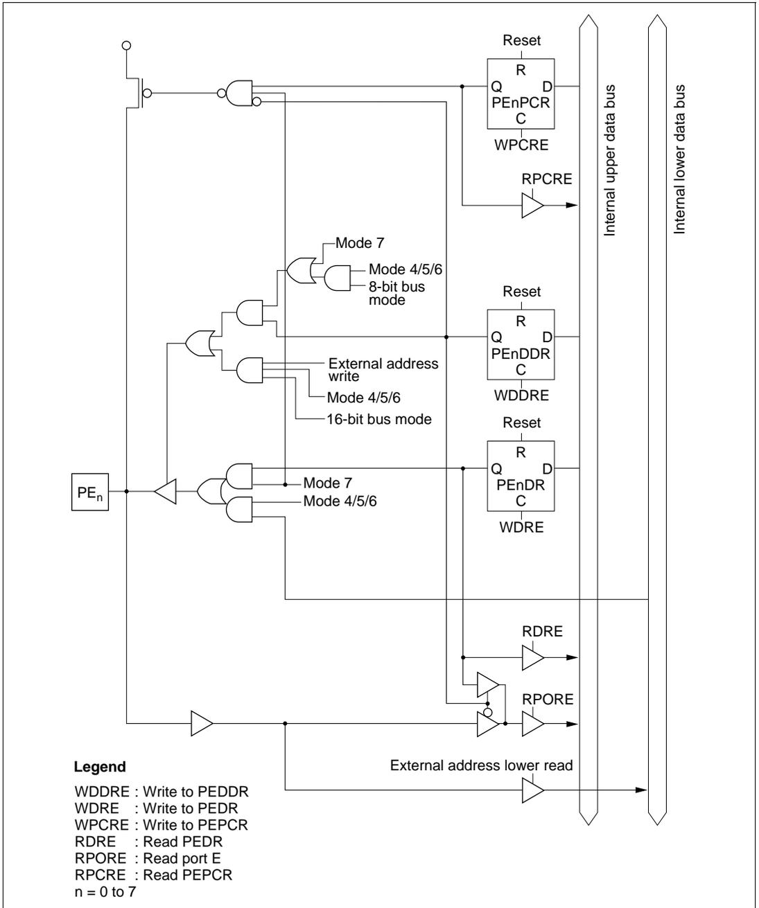
Figure C-11 Port E Block Diagram (Pin  $PE_n$ )
