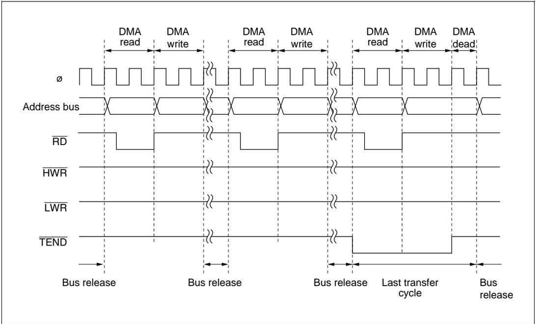
**Figure 7-19 Example of Short Address Mode Transfer**
