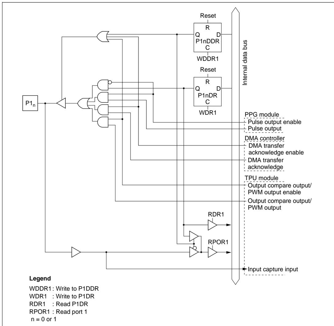
Figure C-1 (a) Port 1 Block Diagram (Pins P1<sub>0</sub> and P1<sub>1</sub>)
