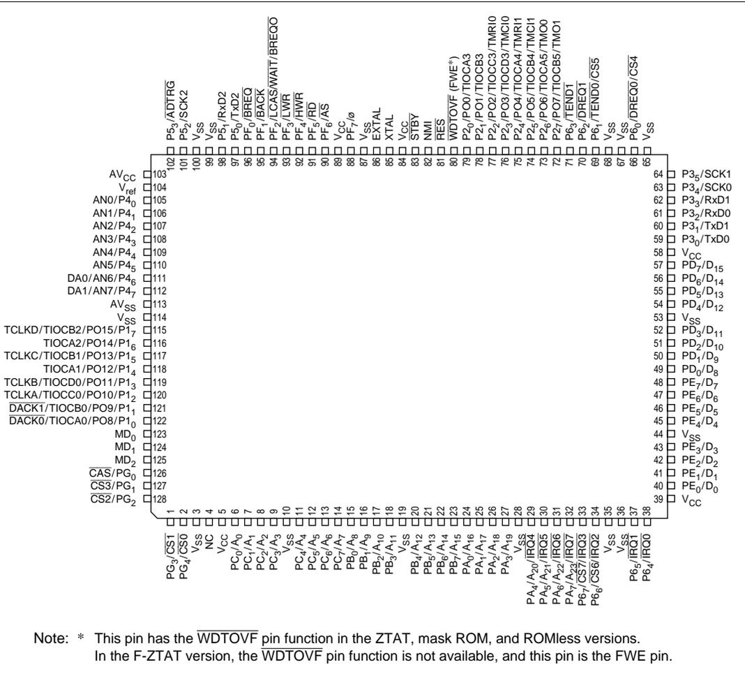
**Figure 1-3 Pin Arrangement (FP-128: Top View)**
