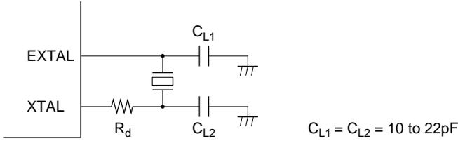
**Figure 20-2 Connection of Crystal Resonator (Example)**
