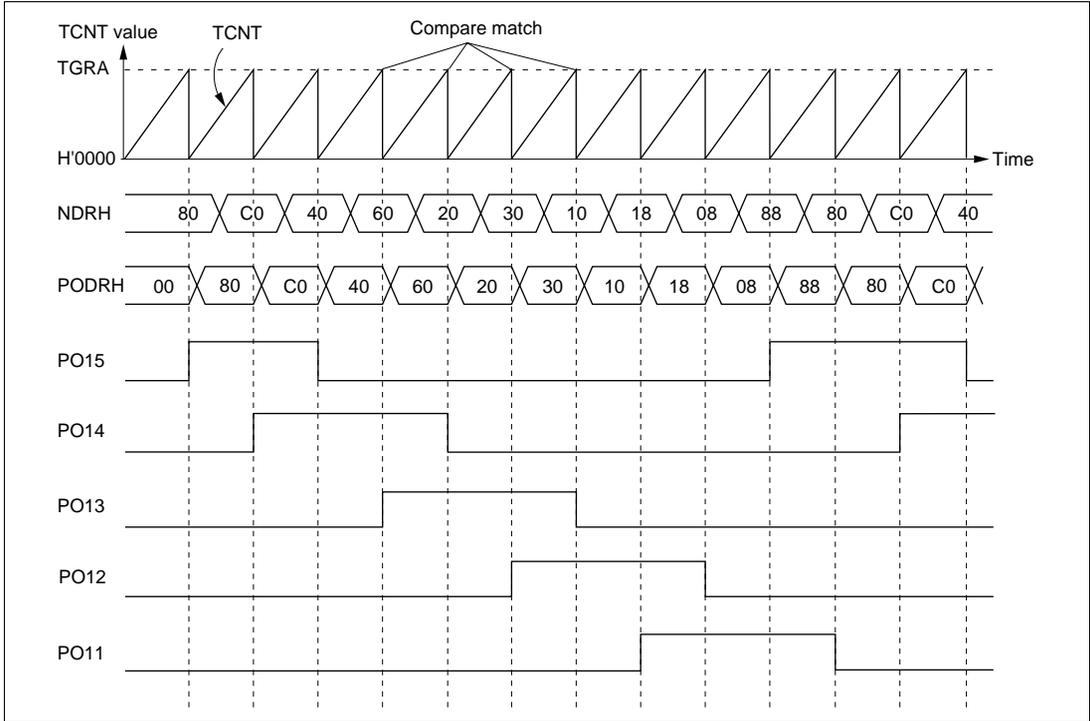
**Figure 11-5 Normal Pulse Output Example (Five-Phase Pulse Output)**
