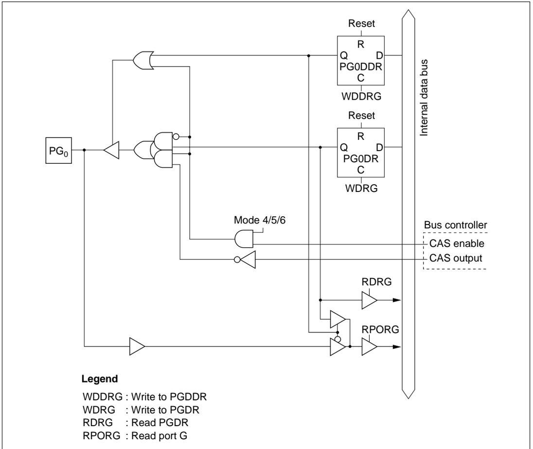
Figure C-13 (a) Port G Block Diagram (Pin  $PG_0$ )
