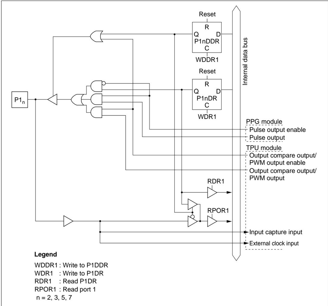
**Figure C-1 (b) Port 1 Block Diagram (Pins P1<sub>2</sub>, P1<sub>3</sub>, P1<sub>5</sub>, and P1<sub>7</sub>)**
