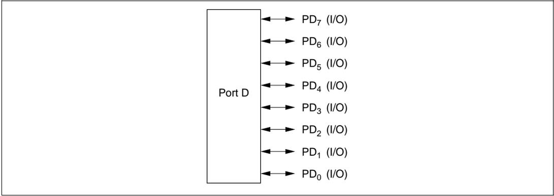
**Figure 9-21 Port D Pin Functions (Mode 7)**
