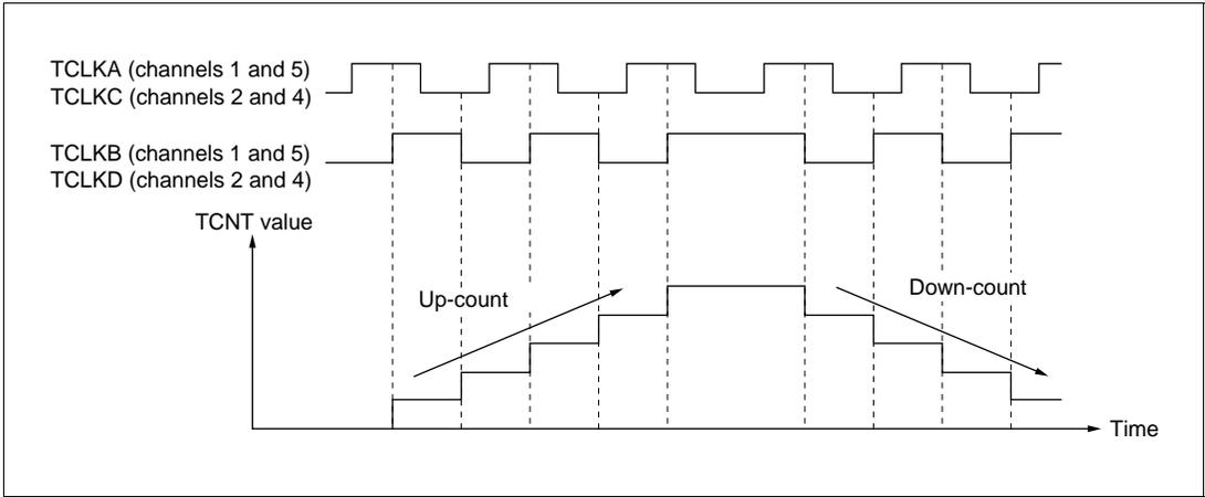
**Figure 10-32 Example of Phase Counting Mode 4 Operation**
