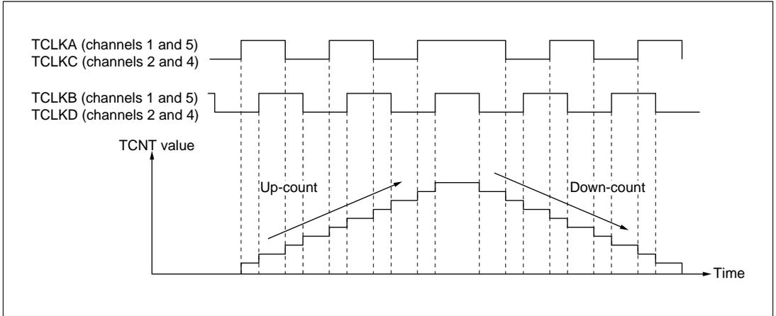
**Figure 10-29 Example of Phase Counting Mode 1 Operation**
