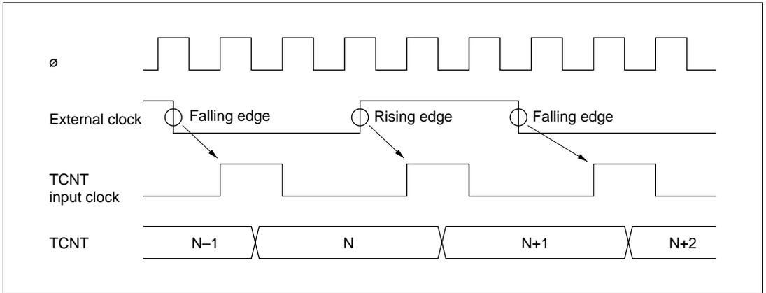
**Figure 10-35 Count Timing in External Clock Operation**
