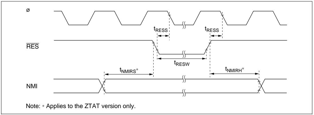
**Figure 22-6 Reset Input Timing**
