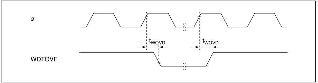
**Figure 22-29 WDT Output Timing**
