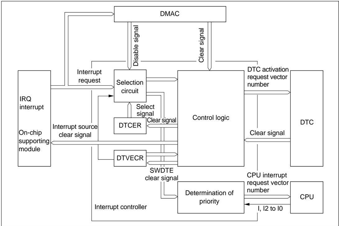
Figure 5-9 Interrupt Control for DTC and DMAC
