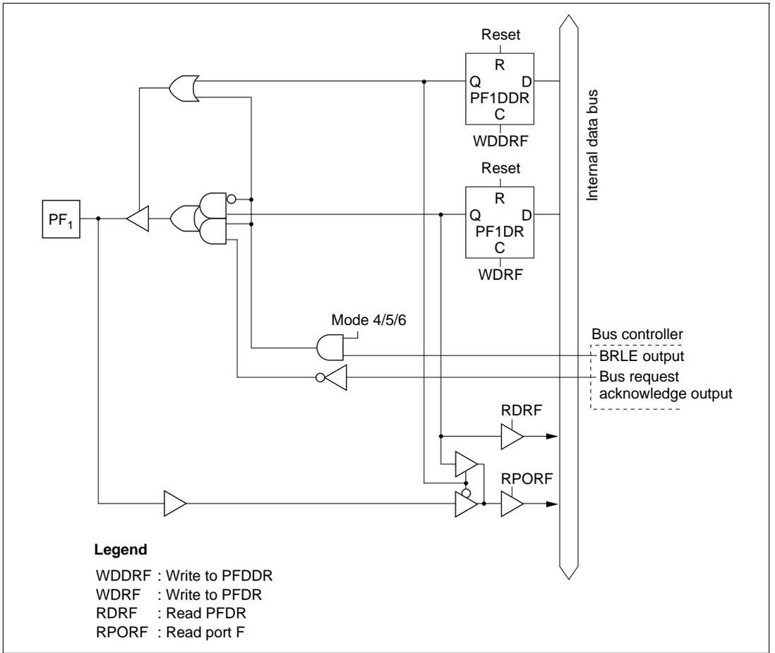
**Figure C-12 (b) Port F Block Diagram (Pin PF<sub>1</sub>)**
