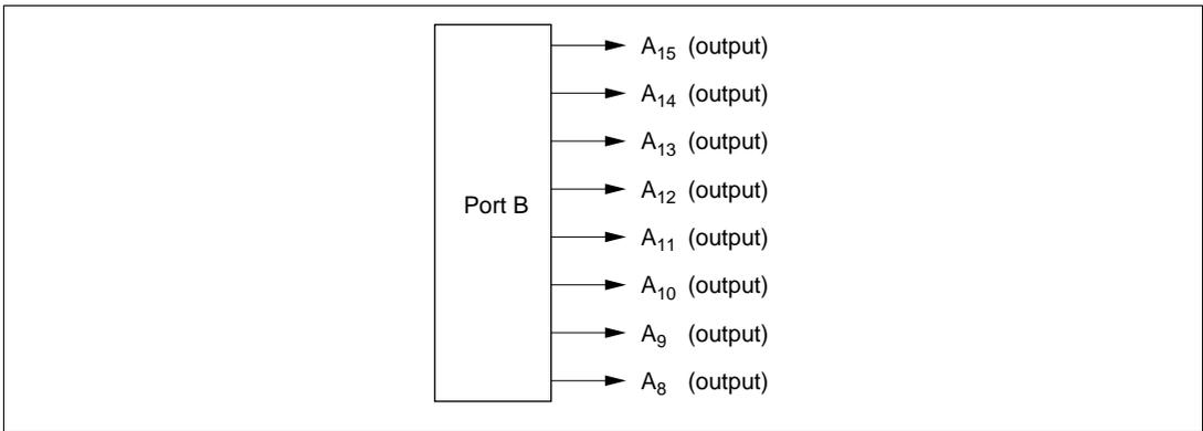
**Figure 9-12 Port B Pin Functions (Modes 4 and 5)**
