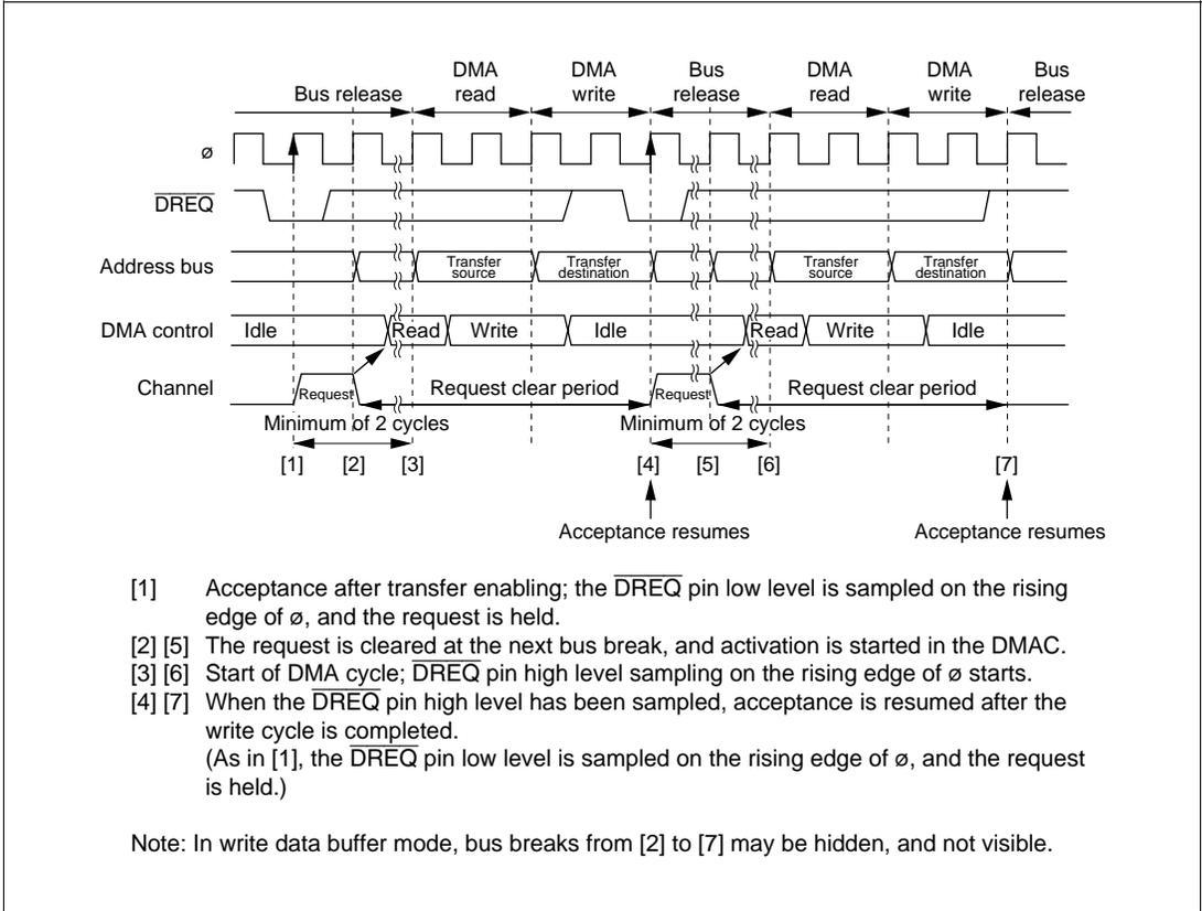
**Figure 7-23 Example of DREQ Pin Falling Edge Activated Normal Mode Transfer**
