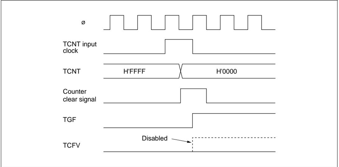
**Figure 10-56** Contention between Overflow and Counter Clearing
