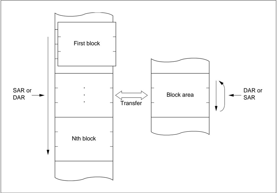
**Figure 8-8 Memory Mapping in Block Transfer Mode**
