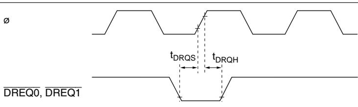
**Figure 22-21 DMAC  $\overline{\text{DREQ}}$  Input Timing**
