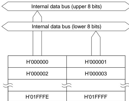
**Figure 19-1 Block Diagram of ROM**
