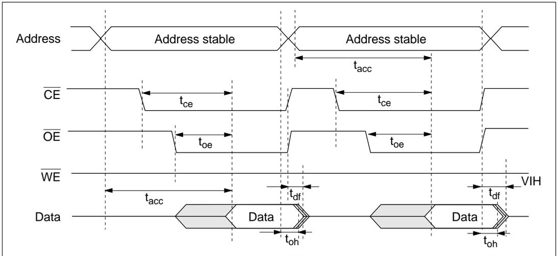
**Figure 19-28 Timing Waveforms for  $\overline{\text{CE}}/\overline{\text{OE}}$  Clocked Read**
