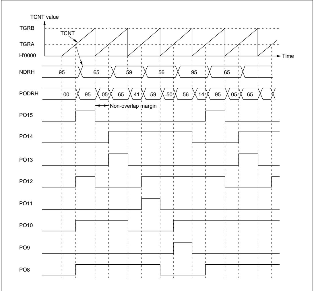
**Figure 11-7 Non-Overlapping Pulse Output Example (Four-Phase Complementary)**
