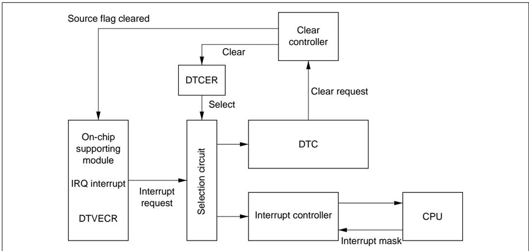
**Figure 8-3 Block Diagram of DTC Activation Source Control**
