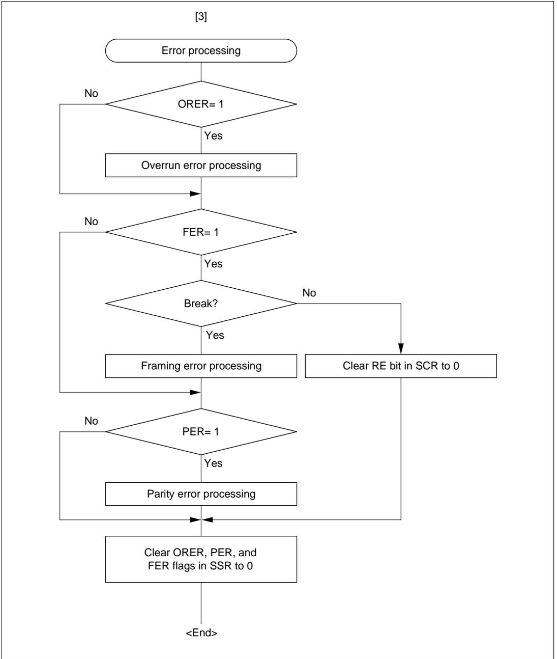
**Figure 14-7 Sample Serial Reception Data Flowchart (cont)**
