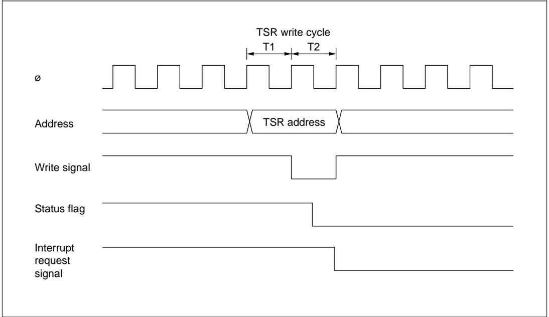
**Figure 10-46 Timing for Status Flag Clearing by CPU**
