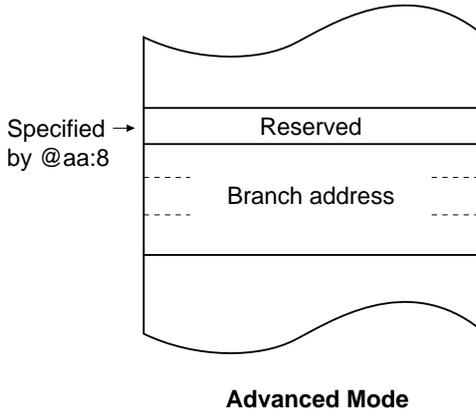
**Figure 2-10 Branch Address Specification in Memory Indirect Mode**
