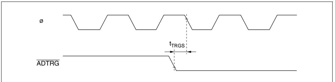
**Figure 22-32 A/D Converter External Trigger Input Timing**
