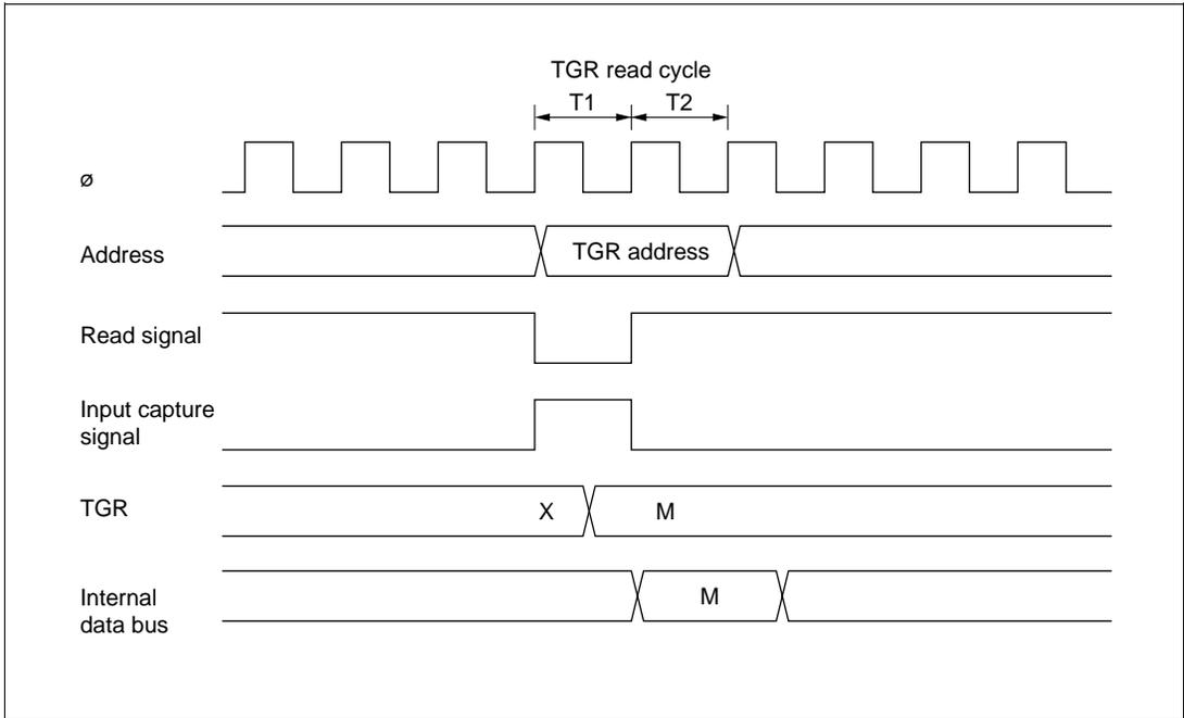
**Figure 10-53 Contention between TGR Read and Input Capture**
