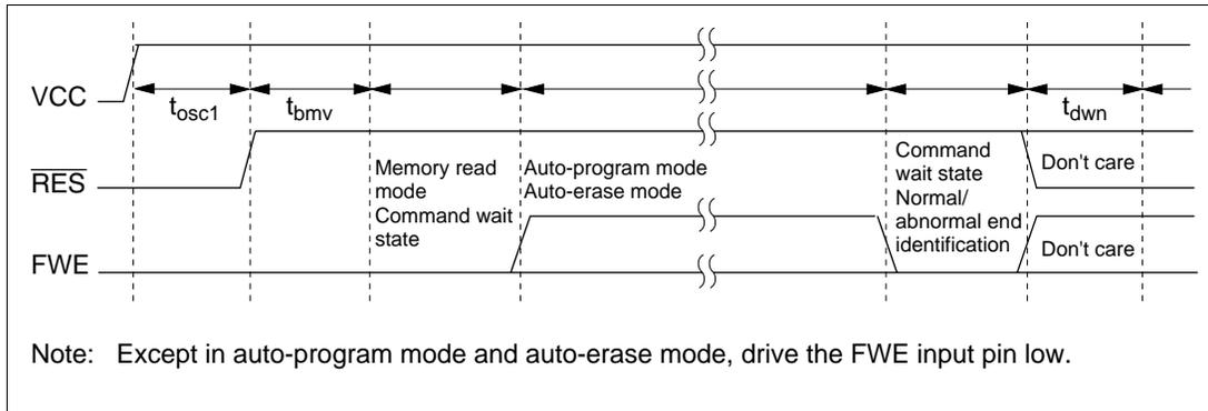
**Figure 19-32 Oscillation Stabilization Time, Writer Mode Setup Time, and Power Supply Fall Sequence**
