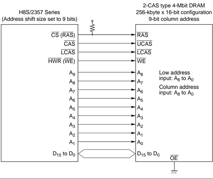
**Figure 6-19 Example of 2-CAS System Connection**
