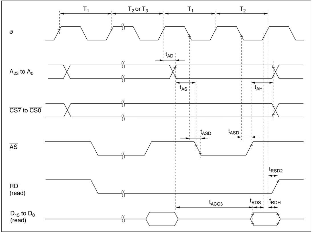
**Figure 22-14 Burst ROM Access Timing (Two-State Access)**
