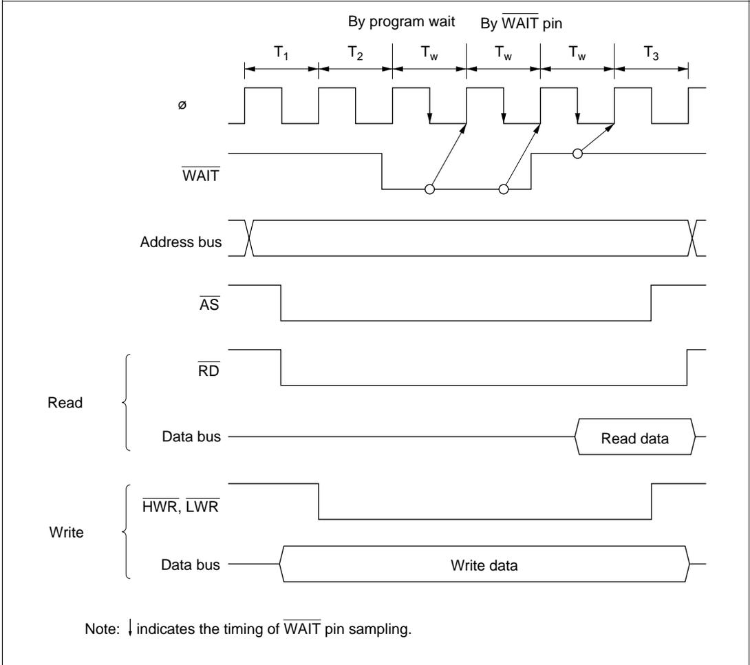
**Figure 6-14 Example of Wait State Insertion Timing**
