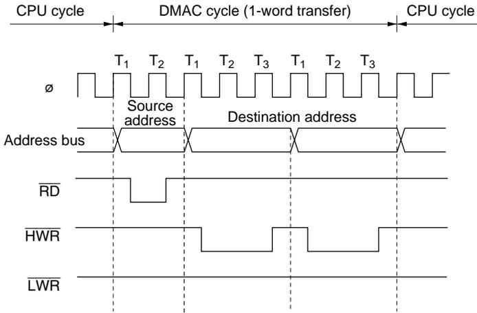
**Figure 7-18 Example of DMA Transfer Bus Timing**
