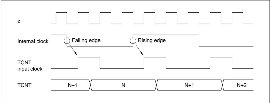
**Figure 10-34 Count Timing in Internal Clock Operation**
