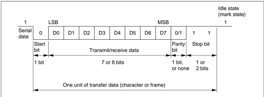
**Figure 14-2 Data Format in Asynchronous Communication**
