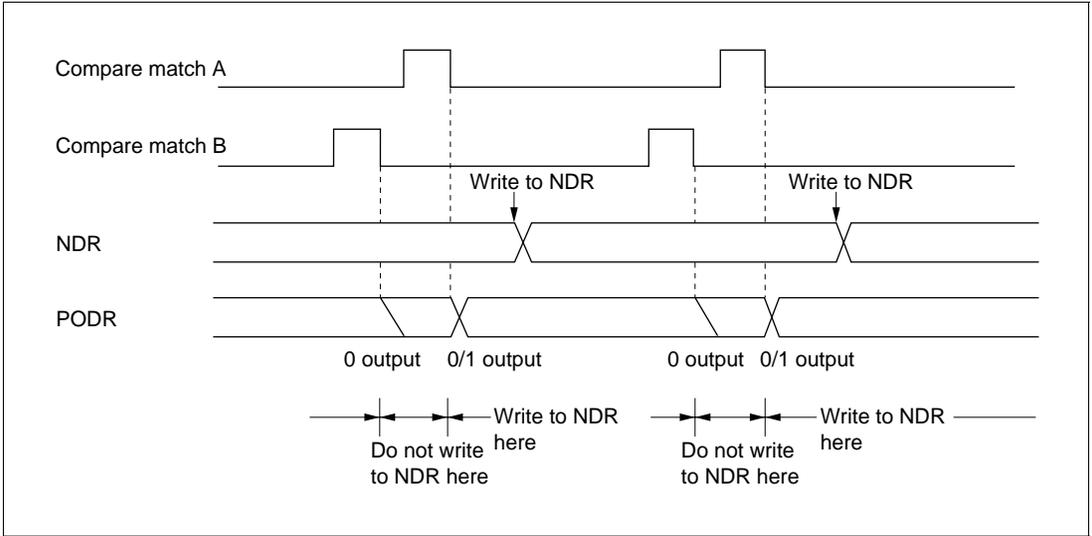
**Figure 11-11 Non-Overlapping Operation and NDR Write Timing**
