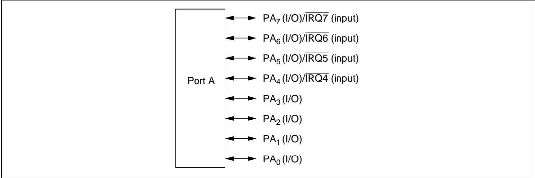
**Figure 9-8 Port A Pin Functions (Mode 7)**
