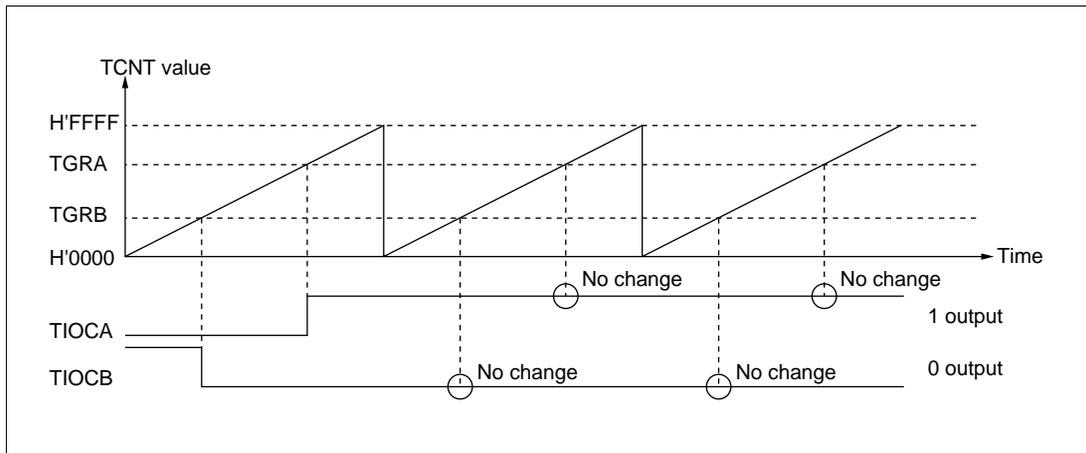
**Figure 10-10 Example of 0 Output/1 Output Operation**
