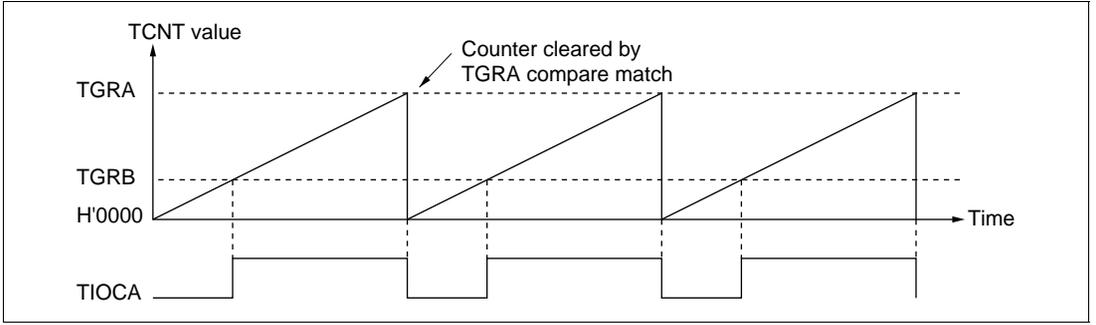
**Figure 10-25 Example of PWM Mode Operation (1)**
