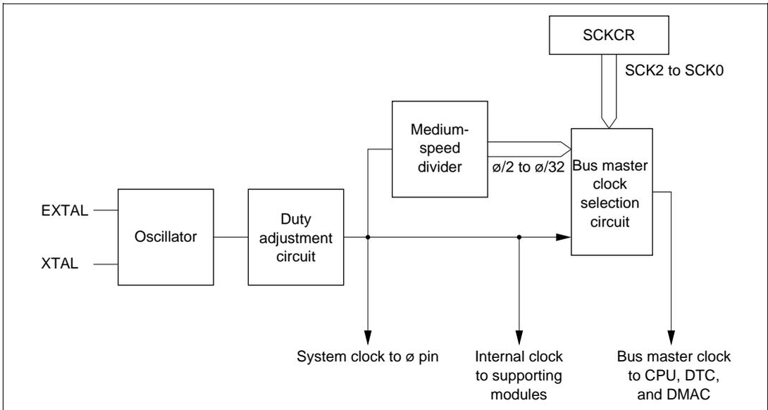
**Figure 20-1 Block Diagram of Clock Pulse Generator**
