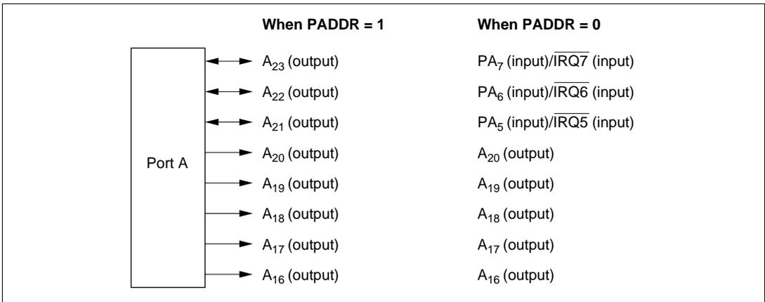
**Figure 9-9 Port A Pin Functions (Modes 4 and 5)**
