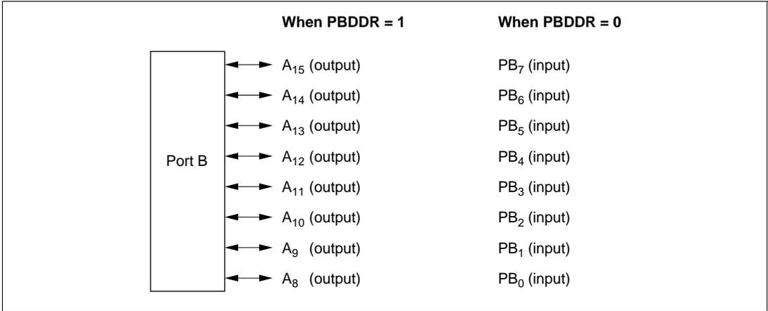
**Figure 9-13 Port B Pin Functions (Modes 6)**
