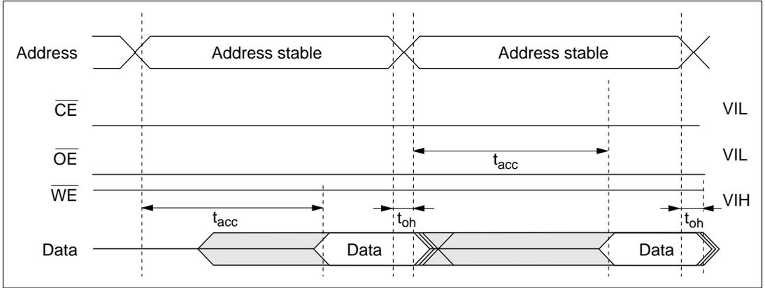
**Figure 19-27 Timing Waveforms for  $\overline{\text{CE}}/\overline{\text{OE}}$  Enable State Read**
