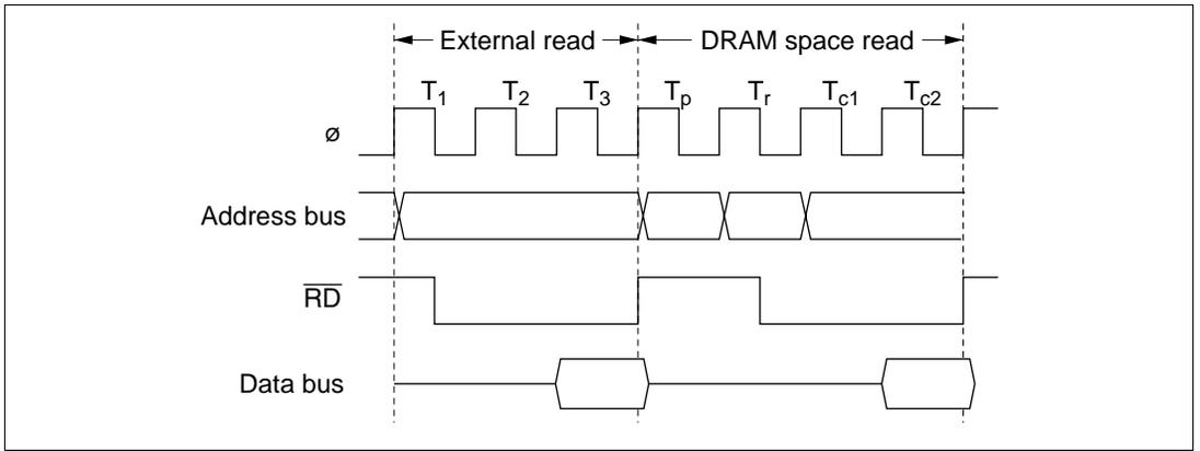
**Figure 6-34 Example of DRAM Access after External Read**
