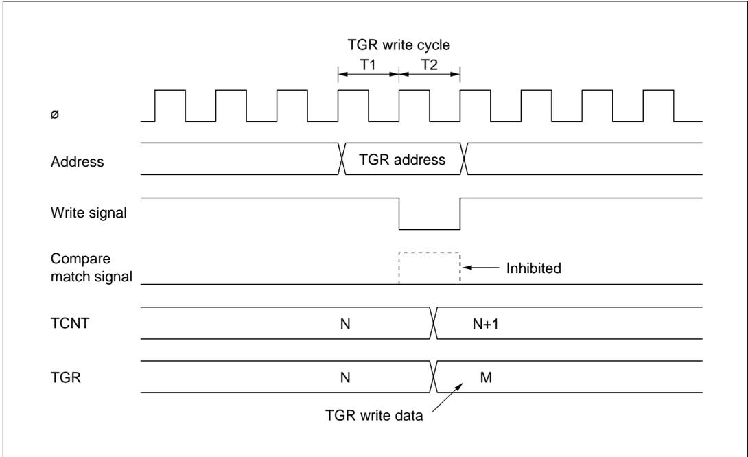
**Figure 10-51 Contention between TGR Write and Compare Match**
