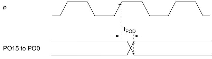
**Figure 22-23 PPG Output Timing**
