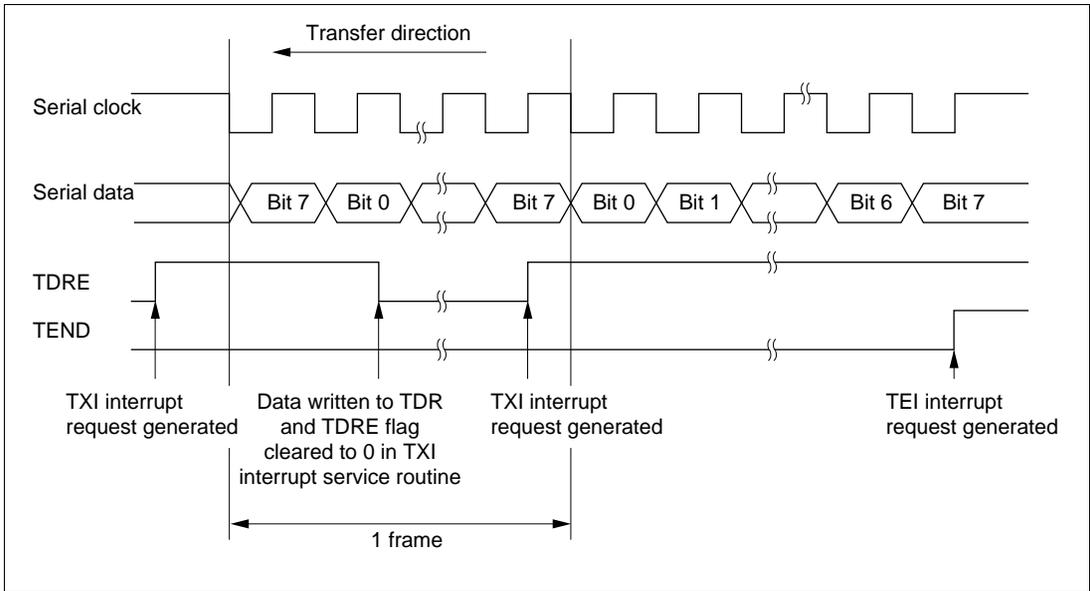
**Figure 14-17 Example of SCI Operation in Transmission**
