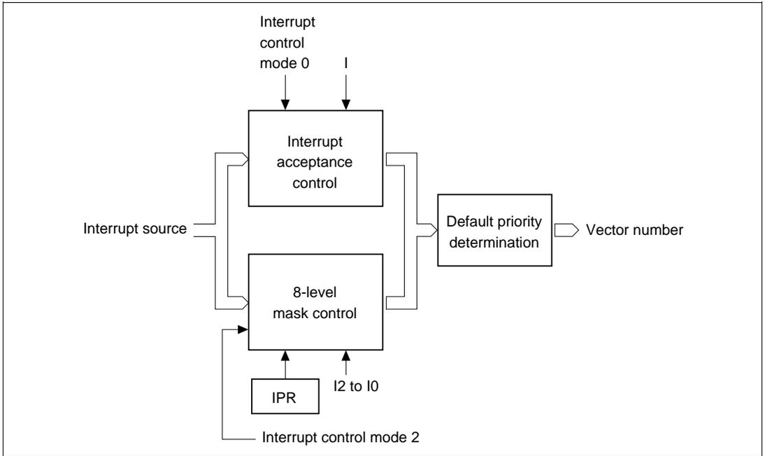
**Figure 5-4 Block Diagram of Interrupt Control Operation**
