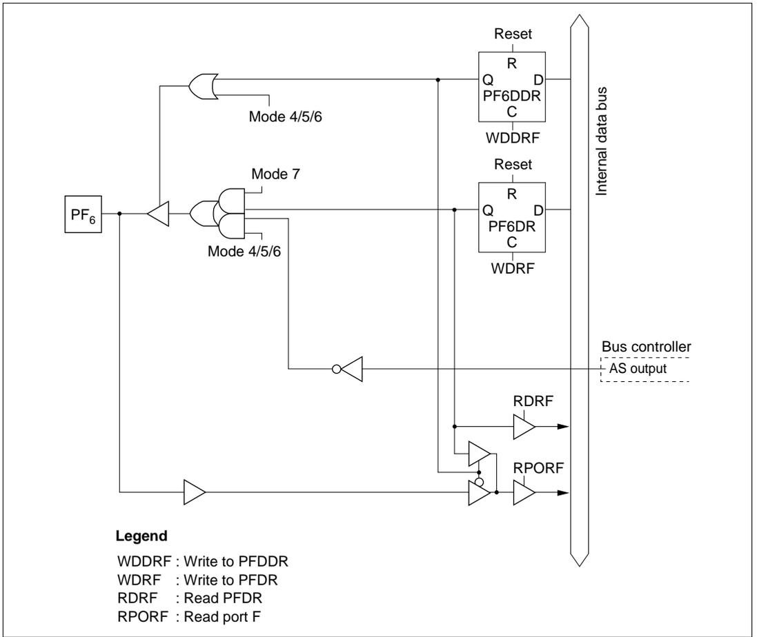
**Figure C-12 (g) Port F Block Diagram (Pin PF<sub>6</sub>)**
