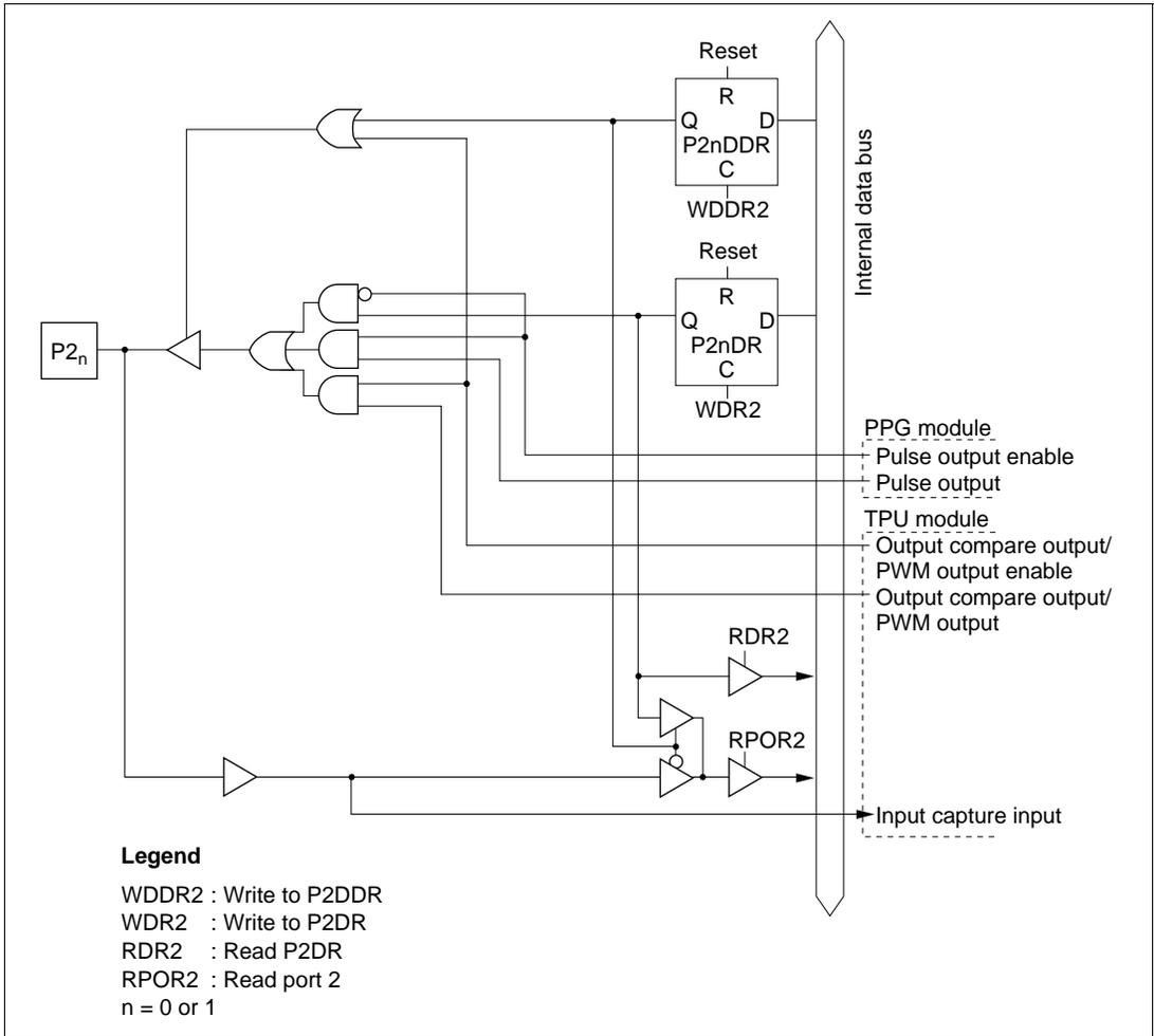
Figure C-2 (a) Port 2 Block Diagram (Pins P2<sub>0</sub> and P2<sub>1</sub>)
