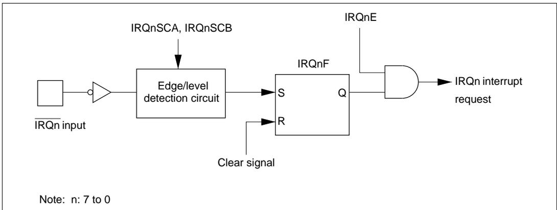
Figure 5-2 Block Diagram of Interrupts IRQ7 to IRQ0
