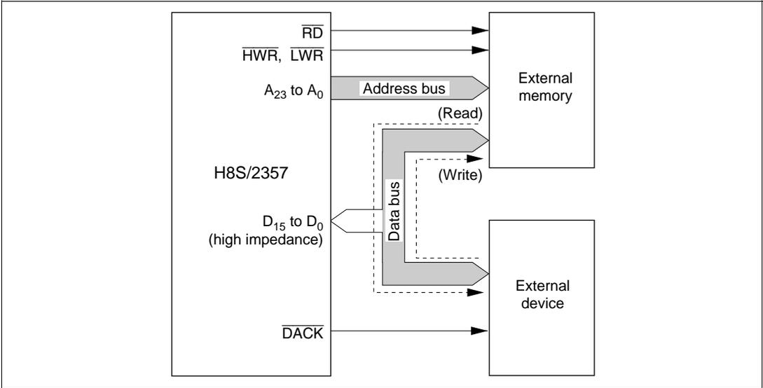
**Figure 7-17 Data Bus in Single Address Mode**
