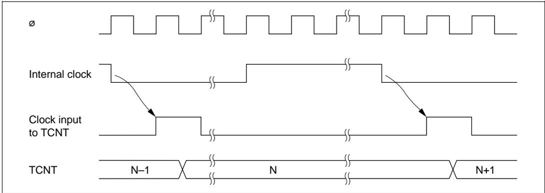
**Figure 12-2 Count Timing for Internal Clock Input**
