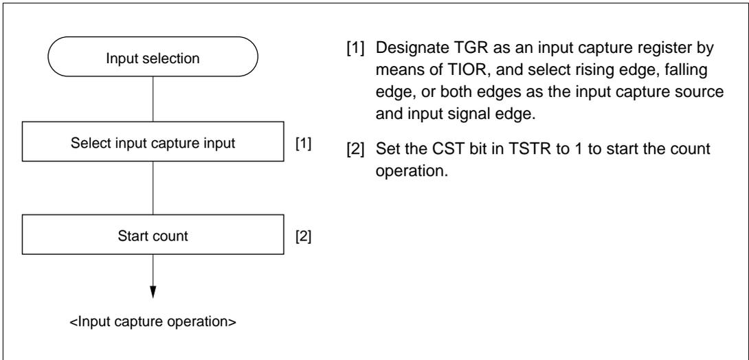
**Figure 10-12 Example of Input Capture Operation Setting Procedure**
