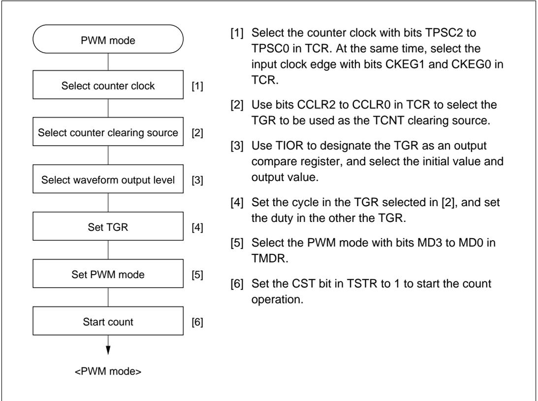
**Figure 10-24 Example of PWM Mode Setting Procedure**
