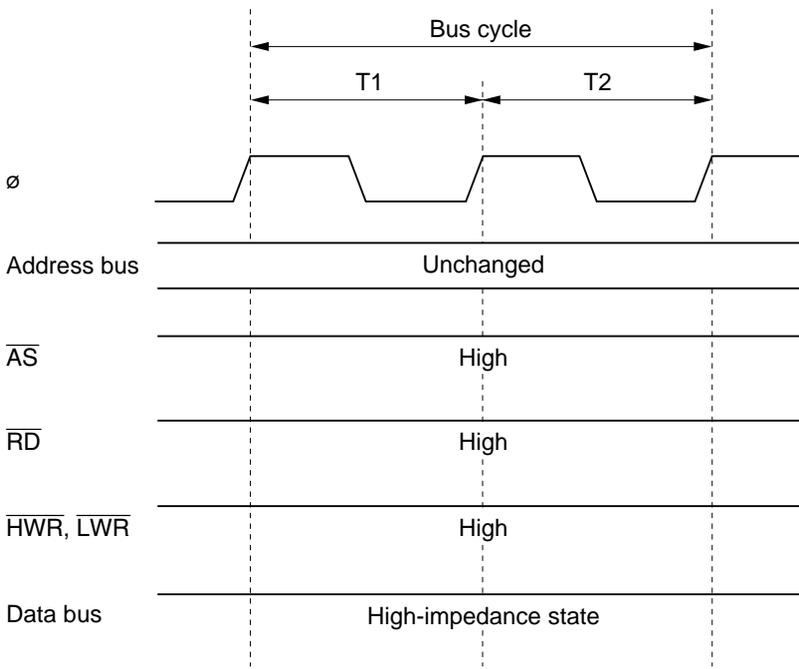
**Figure 2-17 Pin States during On-Chip Supporting Module Access**
