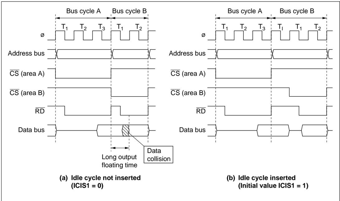
Figure 6-31 Example of Idle Cycle Operation (1)
