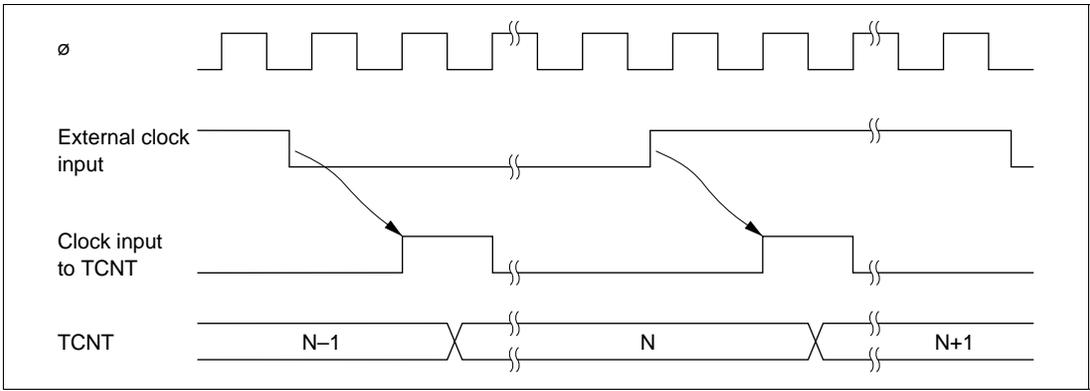
**Figure 12-3 Count Timing for External Clock Input**
