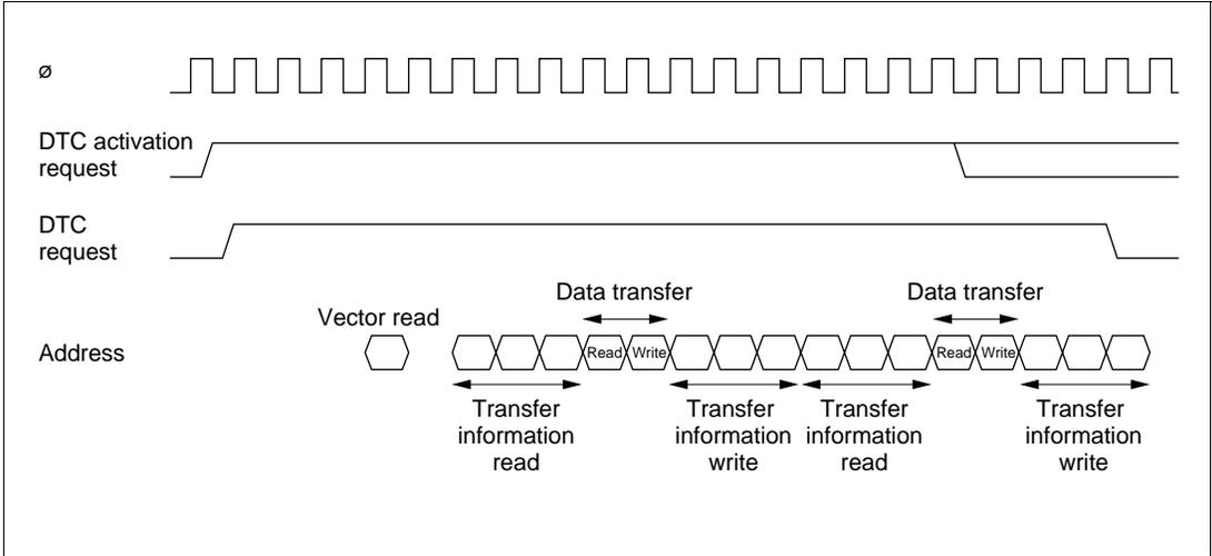
**Figure 8-12 DTC Operation Timing (Example of Chain Transfer)**
