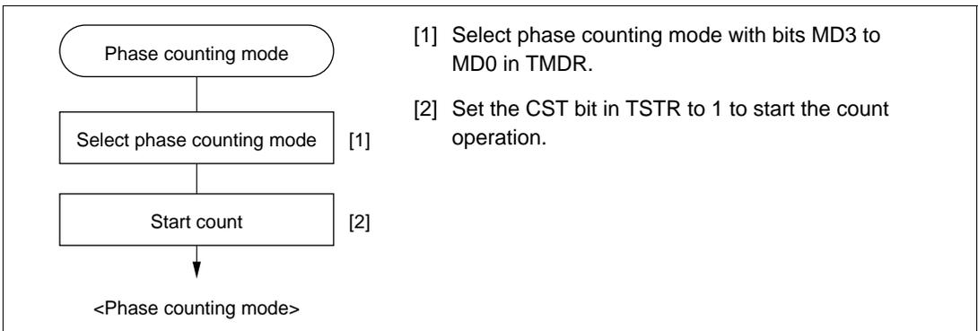
**Figure 10-28 Example of Phase Counting Mode Setting Procedure**
