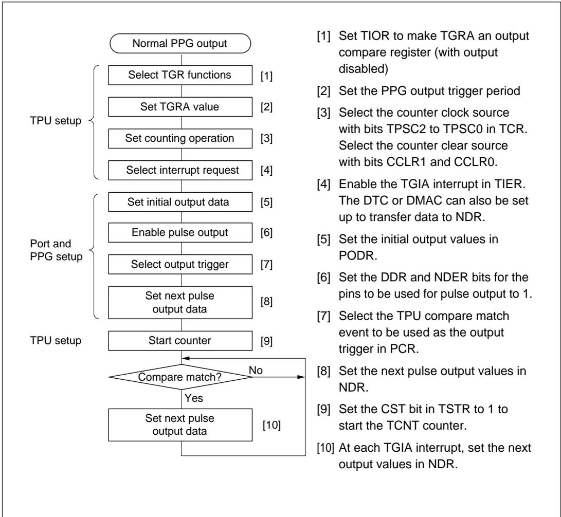
**Figure 11-4 Setup Procedure for Normal Pulse Output (Example)**
