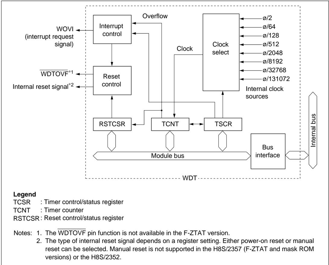
**Figure 13-1 Block Diagram of WDT**
