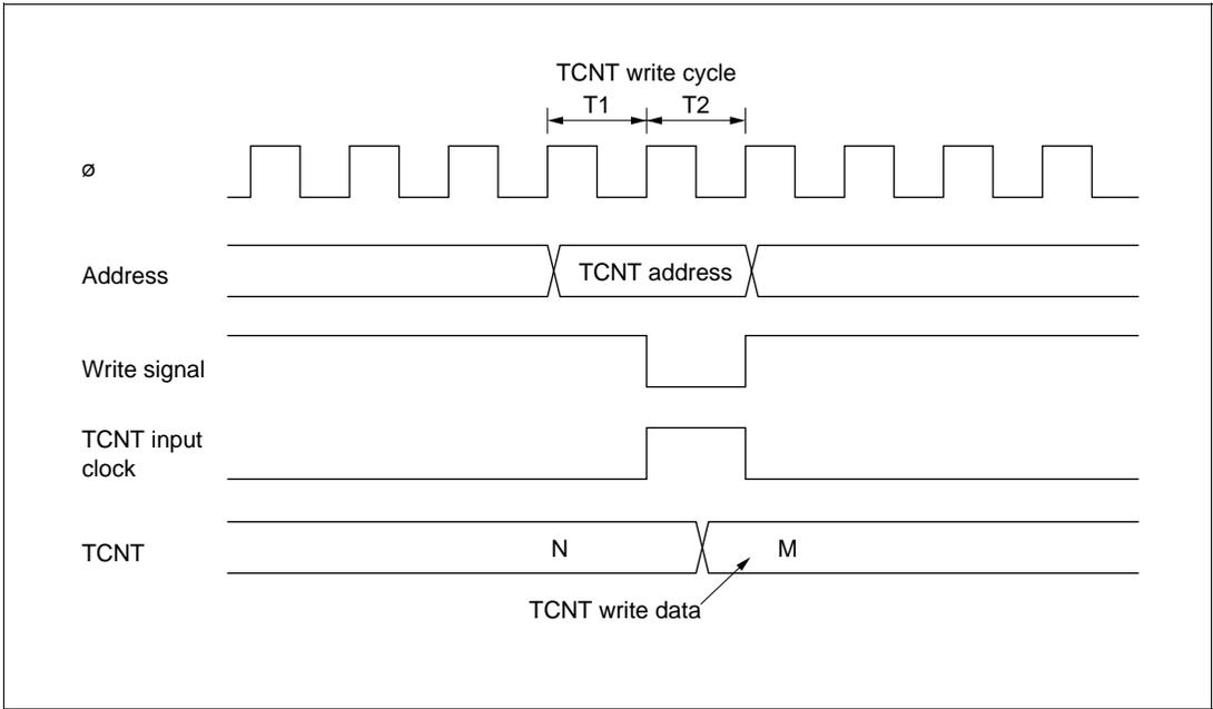
**Figure 10-50 Contention between TCNT Write and Increment Operations**
