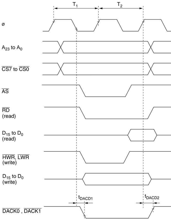
**Figure 22-18 DMAC Single Address Transfer Timing (Two-State Access)**
