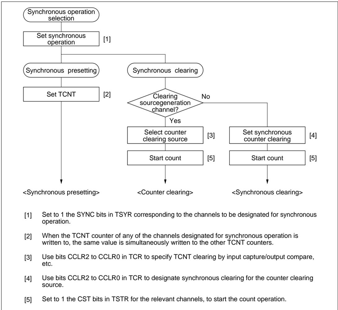
**Figure 10-14 Example of Synchronous Operation Setting Procedure**
