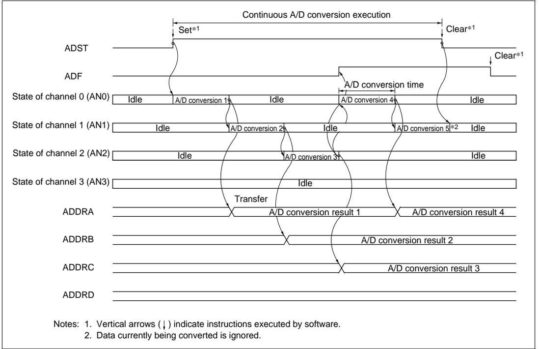
**Figure 16-4 Example of A/D Converter Operation
