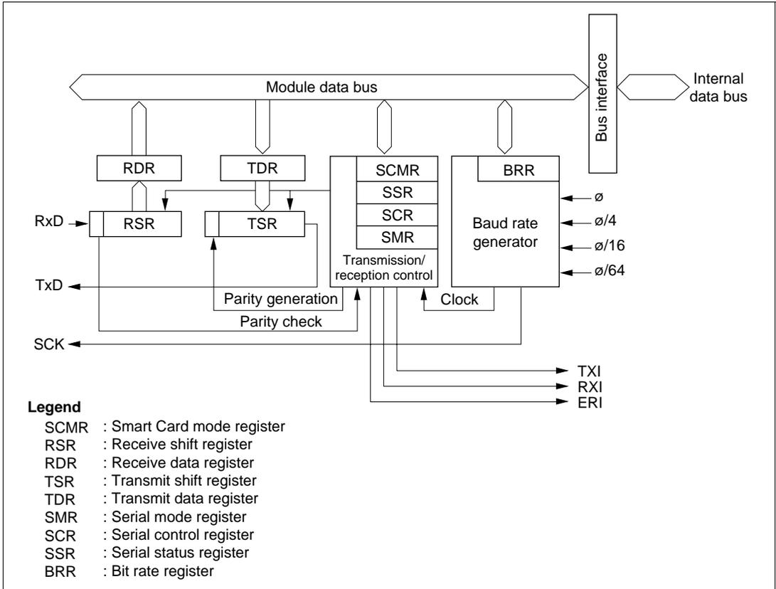
**Figure 15-1 Block Diagram of Smart Card Interface**
