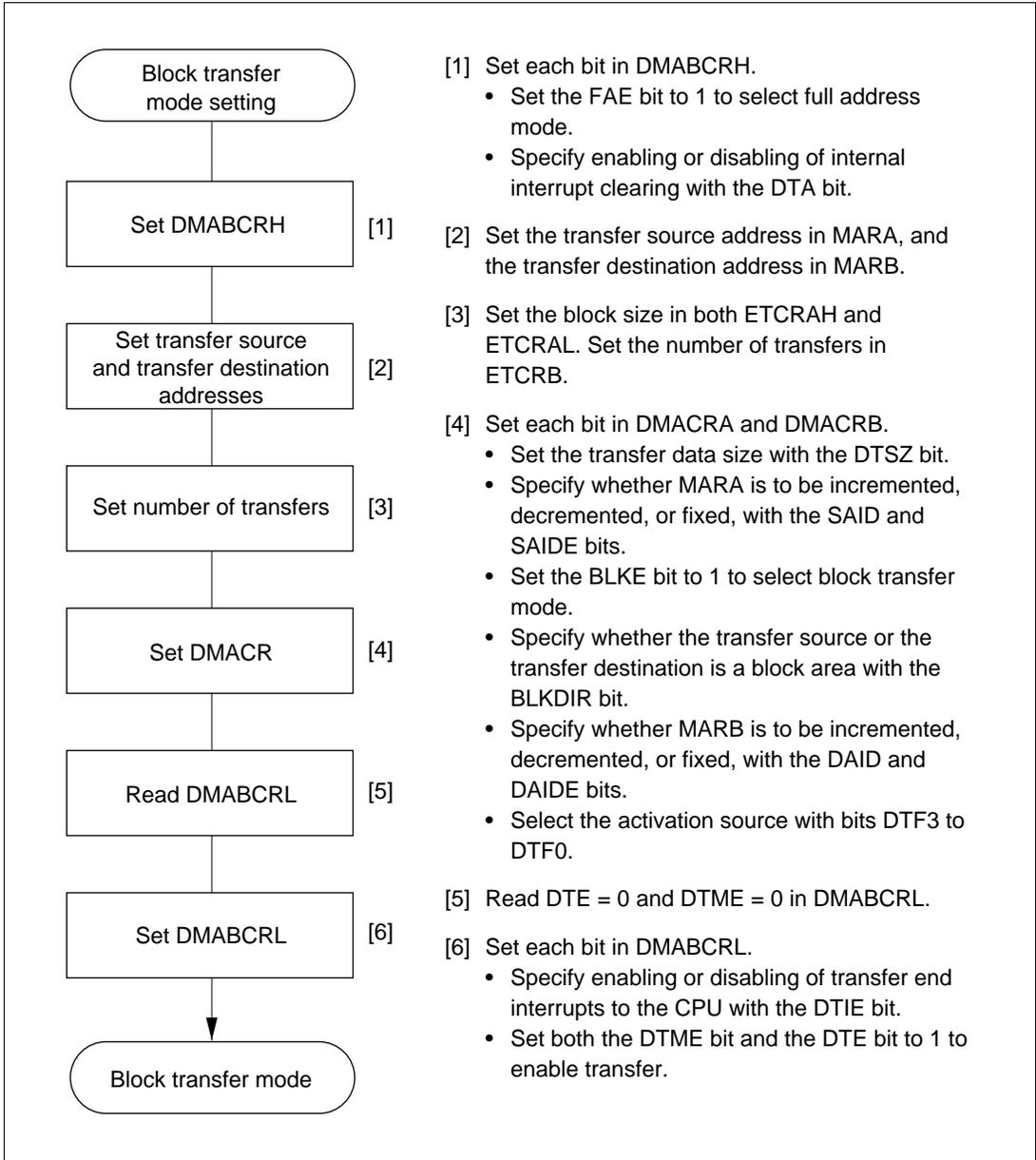
**Figure 7-16 Example of Block Transfer Mode Setting Procedure**
