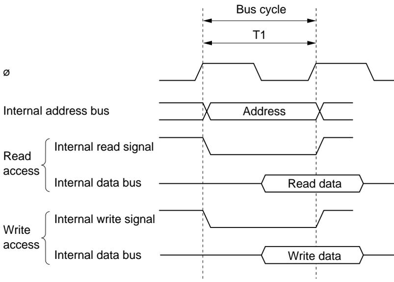
**Figure 2-14 On-Chip Memory Access Cycle**
