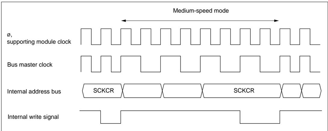
Figure 21-1 Medium-Speed Mode Transition and Clearance Timing
