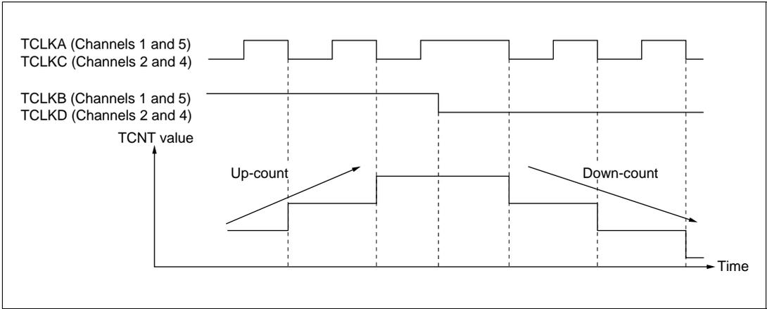
**Figure 10-30 Example of Phase Counting Mode 2 Operation**
