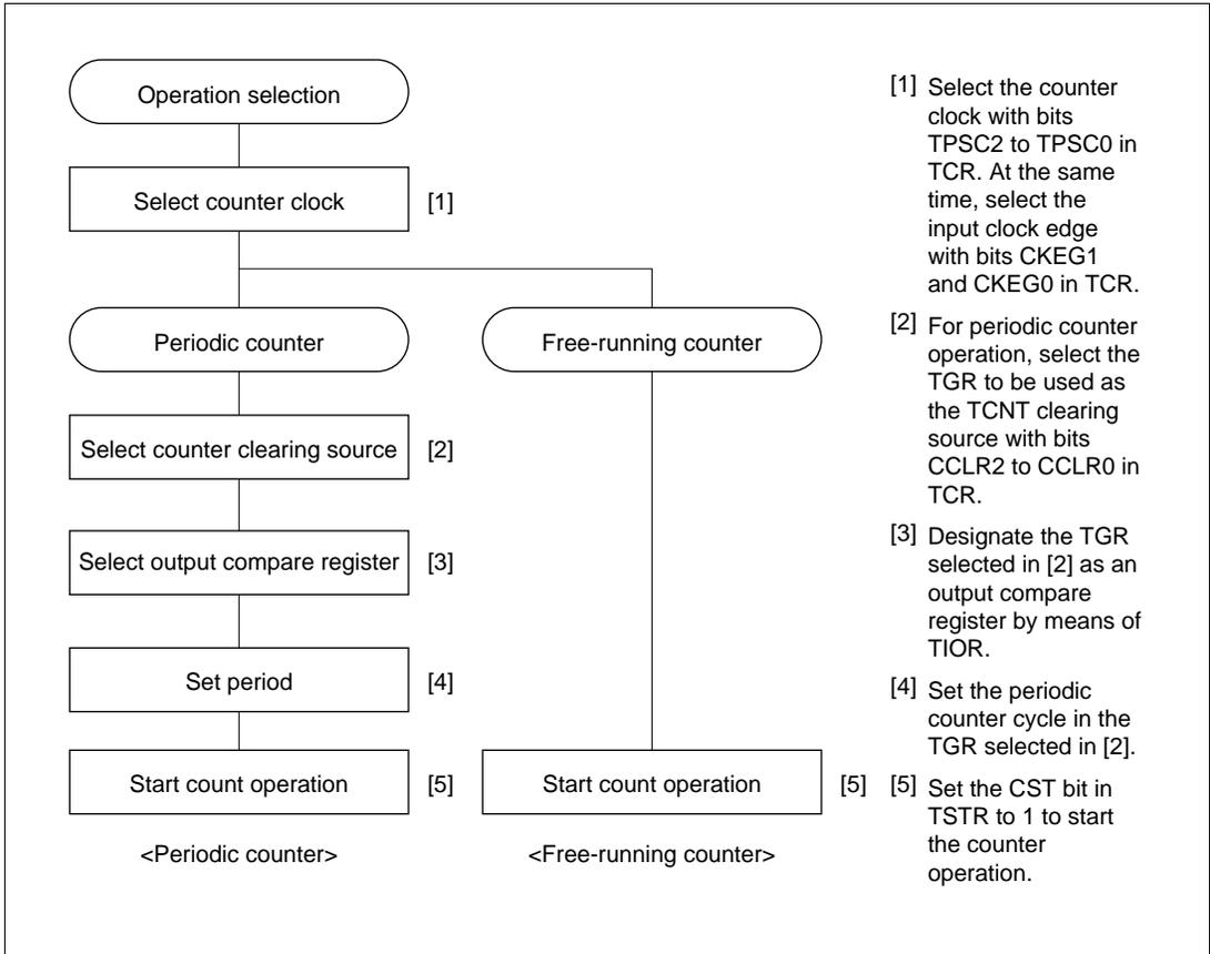
**Figure 10-6 Example of Counter Operation Setting Procedure**
