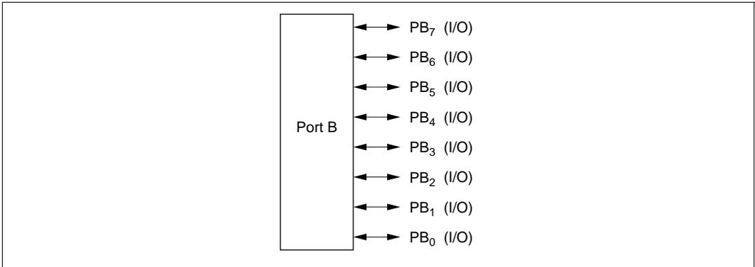
**Figure 9-14 Port B Pin Functions (Mode 7)**
