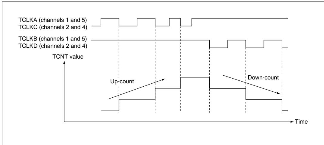
**Figure 10-31 Example of Phase Counting Mode 3 Operation**
