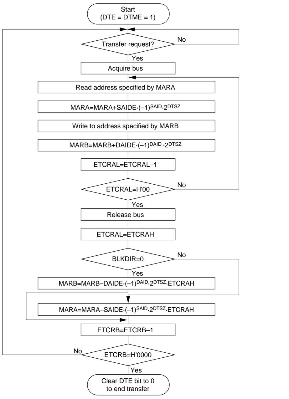
**Figure 7-15 Operation Flow in Block Transfer Mode**
