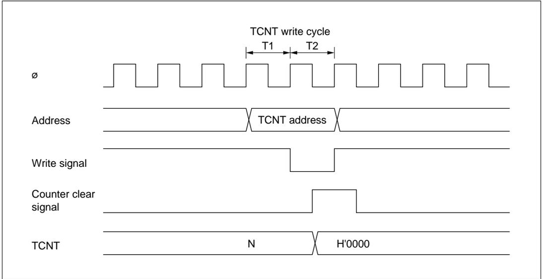
**Figure 10-49 Contention between TCNT Write and Clear Operations**
