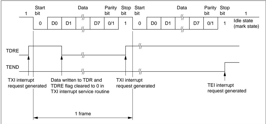
**Figure 14-6 Example of Operation in Transmission in Asynchronous Mode
