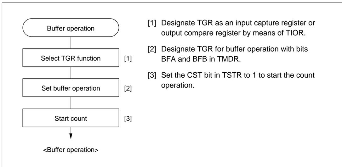
**Figure 10-18 Example of Buffer Operation Setting Procedure**
