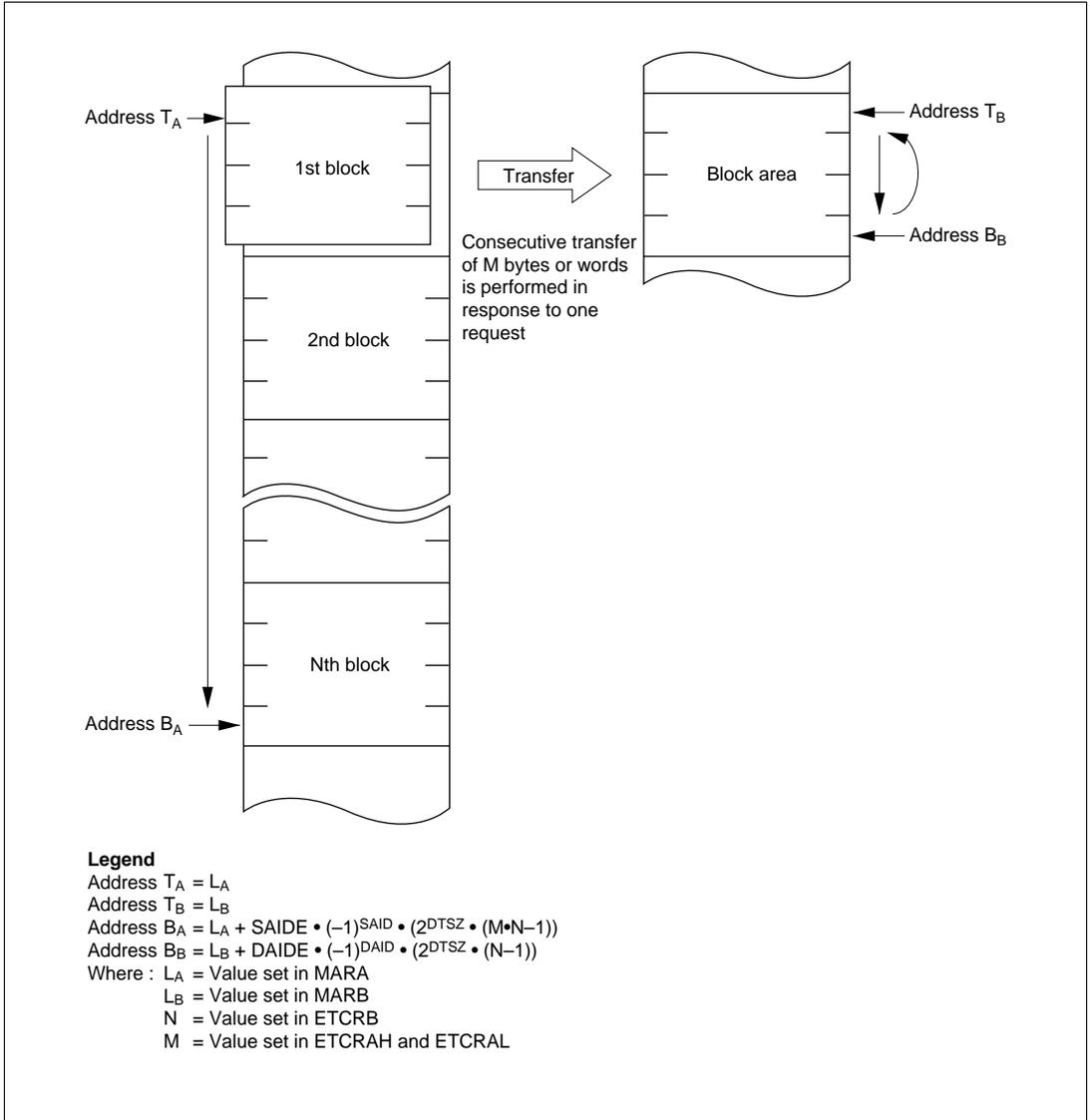
**Figure 7-13 Operation in Block Transfer Mode (BLKDIR = 0)**
