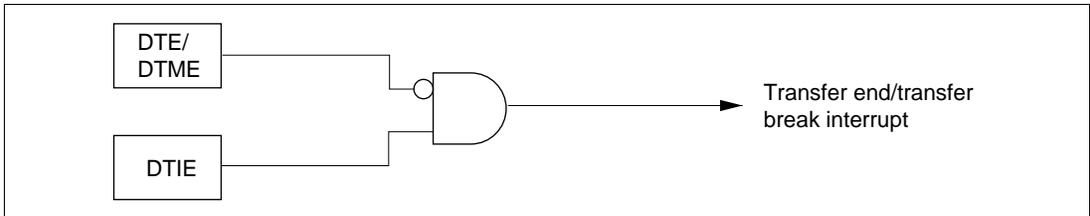
**Figure 7-39 Block Diagram of Transfer End/Transfer Break Interrupt**
