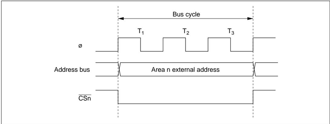
Figure 6-3  $\overline{CSn}$  Signal Output Timing ( $n = 0$  to 7)
