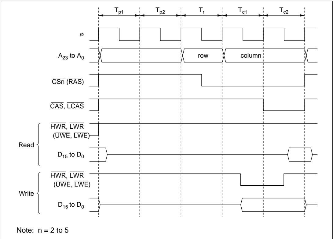
**Figure 6-16 Timing with Two Precharge States (2-WE System)**
