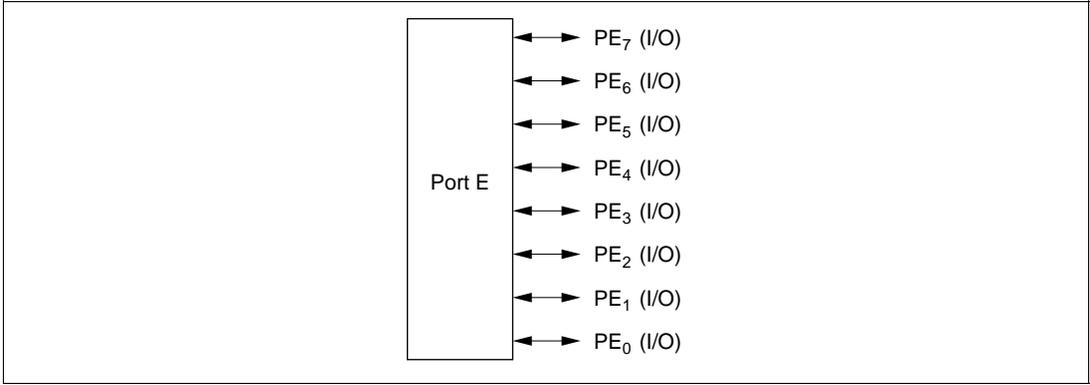
**Figure 9-24 Port E Pin Functions (Mode 7)**
