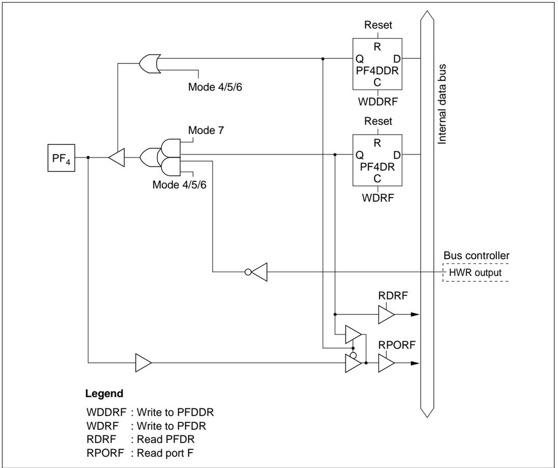
**Figure C-12 (e) Port F Block Diagram (Pin PF<sub>4</sub>)**
