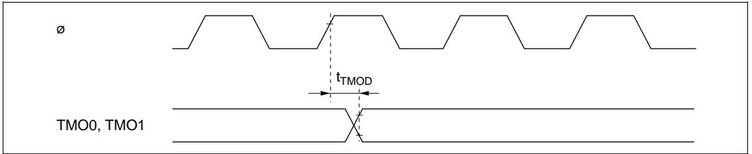
**Figure 22-26 8-Bit Timer Output Timing**
