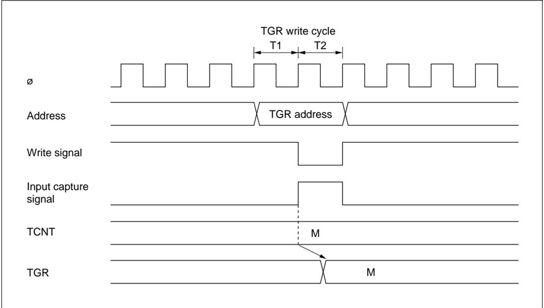
**Figure 10-54** Contention between TGR Write and Input Capture
