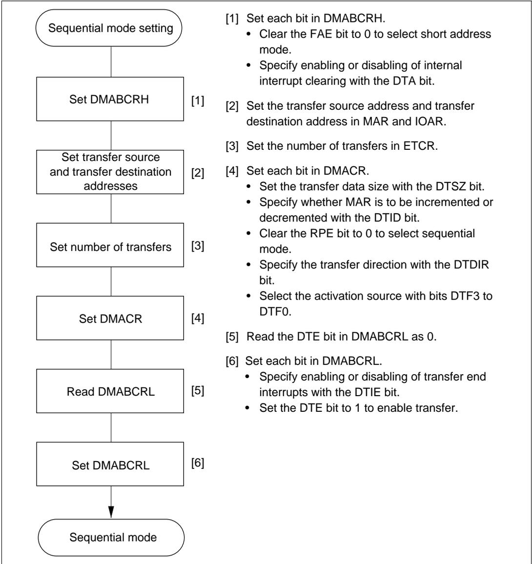
**Figure 7-4 Example of Sequential Mode Setting Procedure**
