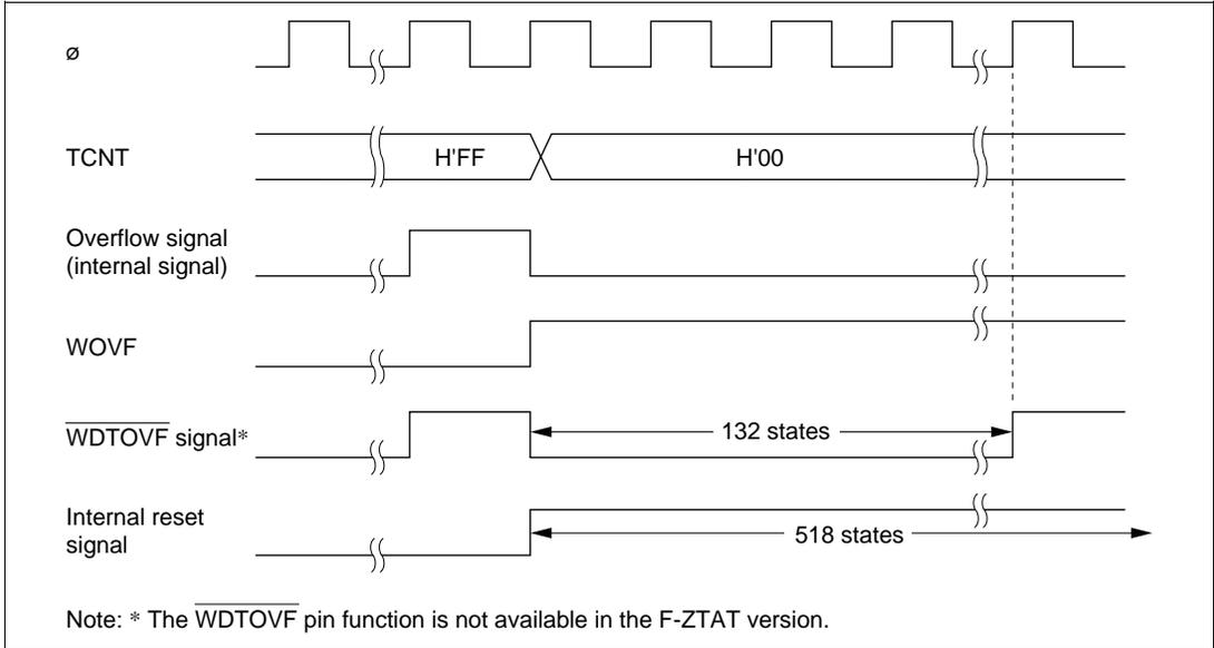
Figure 13-7 Timing of Setting of WOVF
