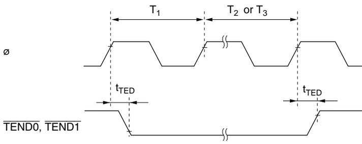
**Figure 22-20 DMAC  $\overline{\text{TEND}}$  Output Timing**
