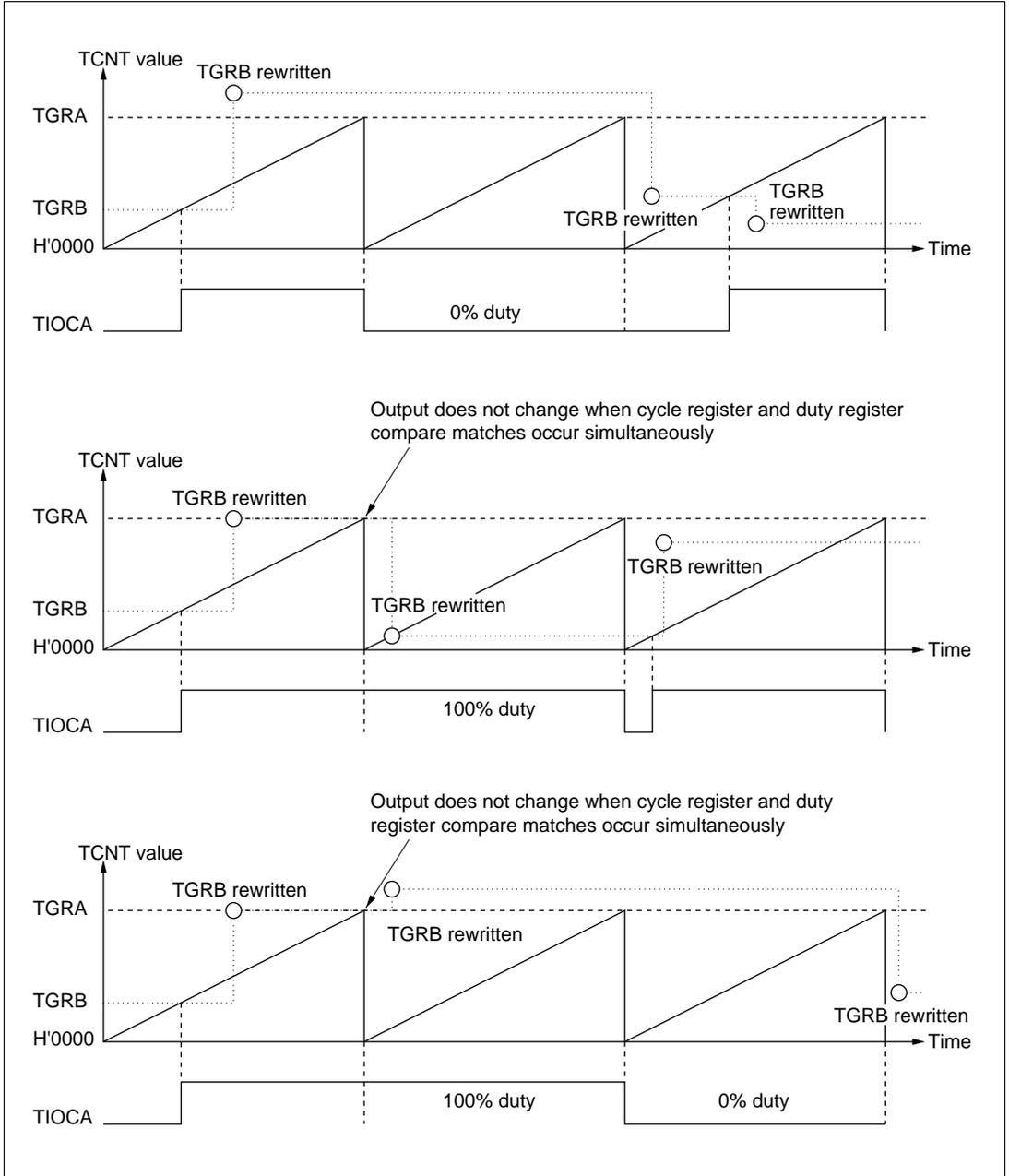
**Figure 10-27 Example of PWM Mode Operation (3)**
