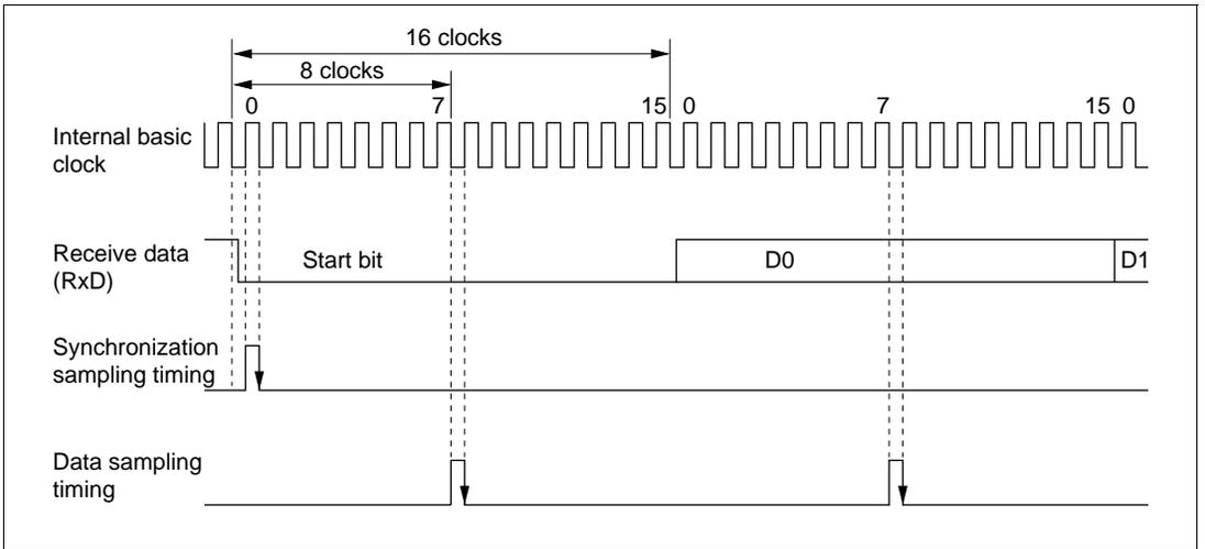
**Figure 14-21 Receive Data Sampling Timing in Asynchronous Mode**
