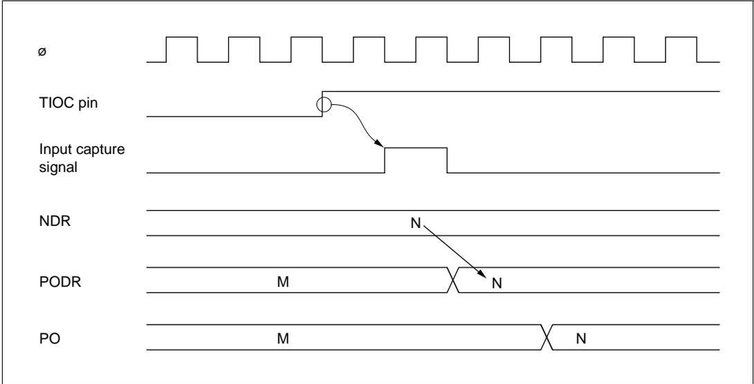
**Figure 11-9 Pulse Output Triggered by Input Capture (Example)**
