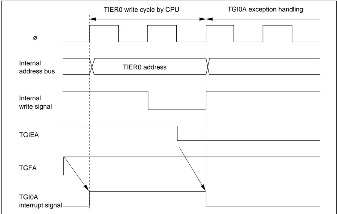
**Figure 5-8 Contention between Interrupt Generation and Disabling**
