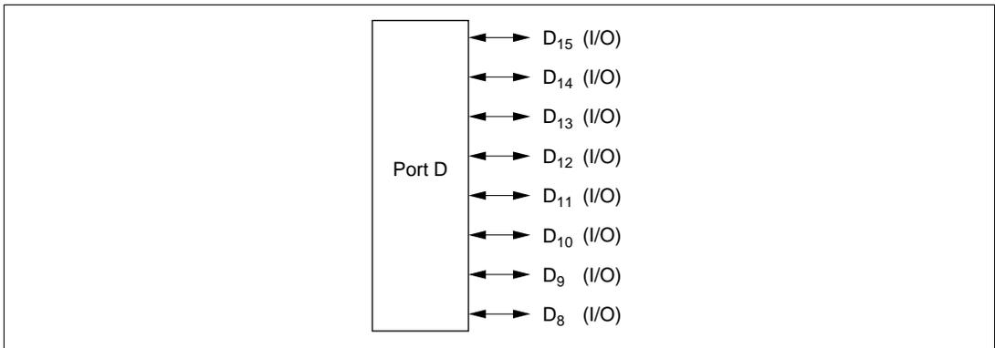
**Figure 9-20 Port D Pin Functions (Modes 4, 5, and 6)**
