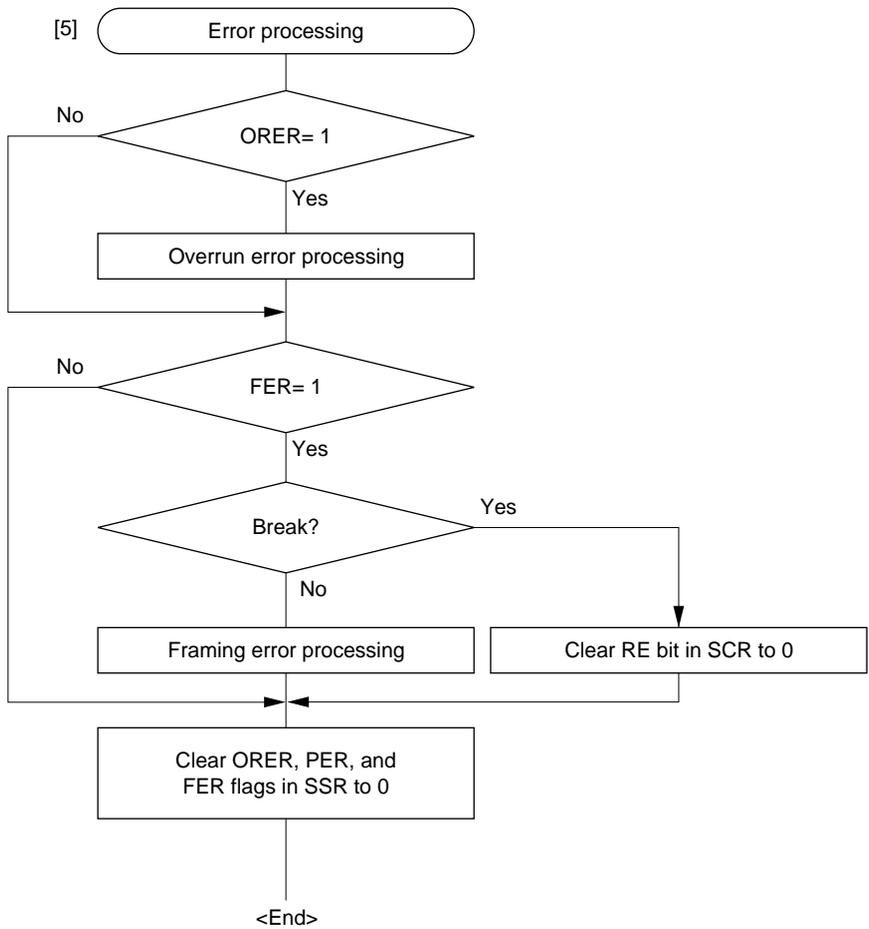
**Figure 14-12 Sample Multiprocessor Serial Reception Flowchart (cont)**
