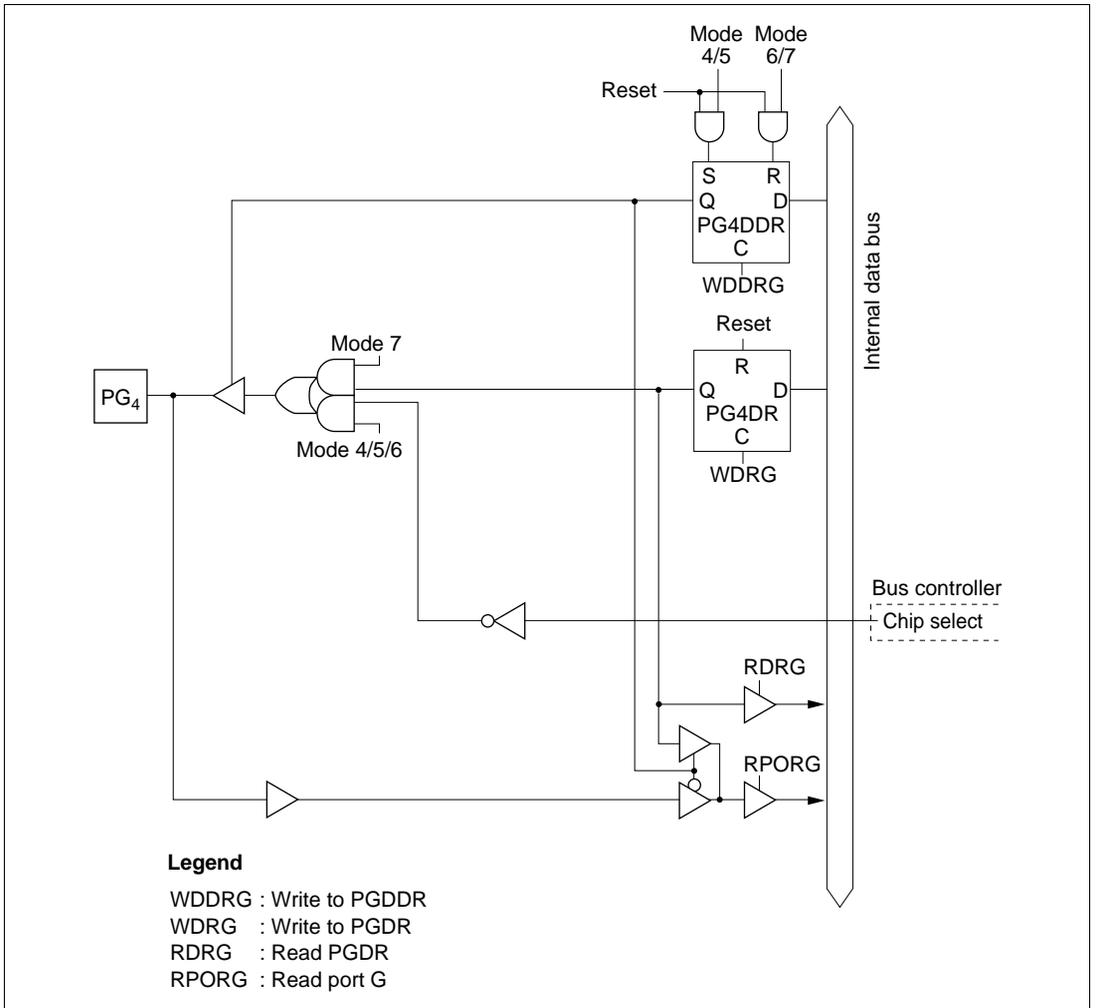
**Figure C-13 (c) Port G Block Diagram (Pin PG<sub>4</sub>)**
