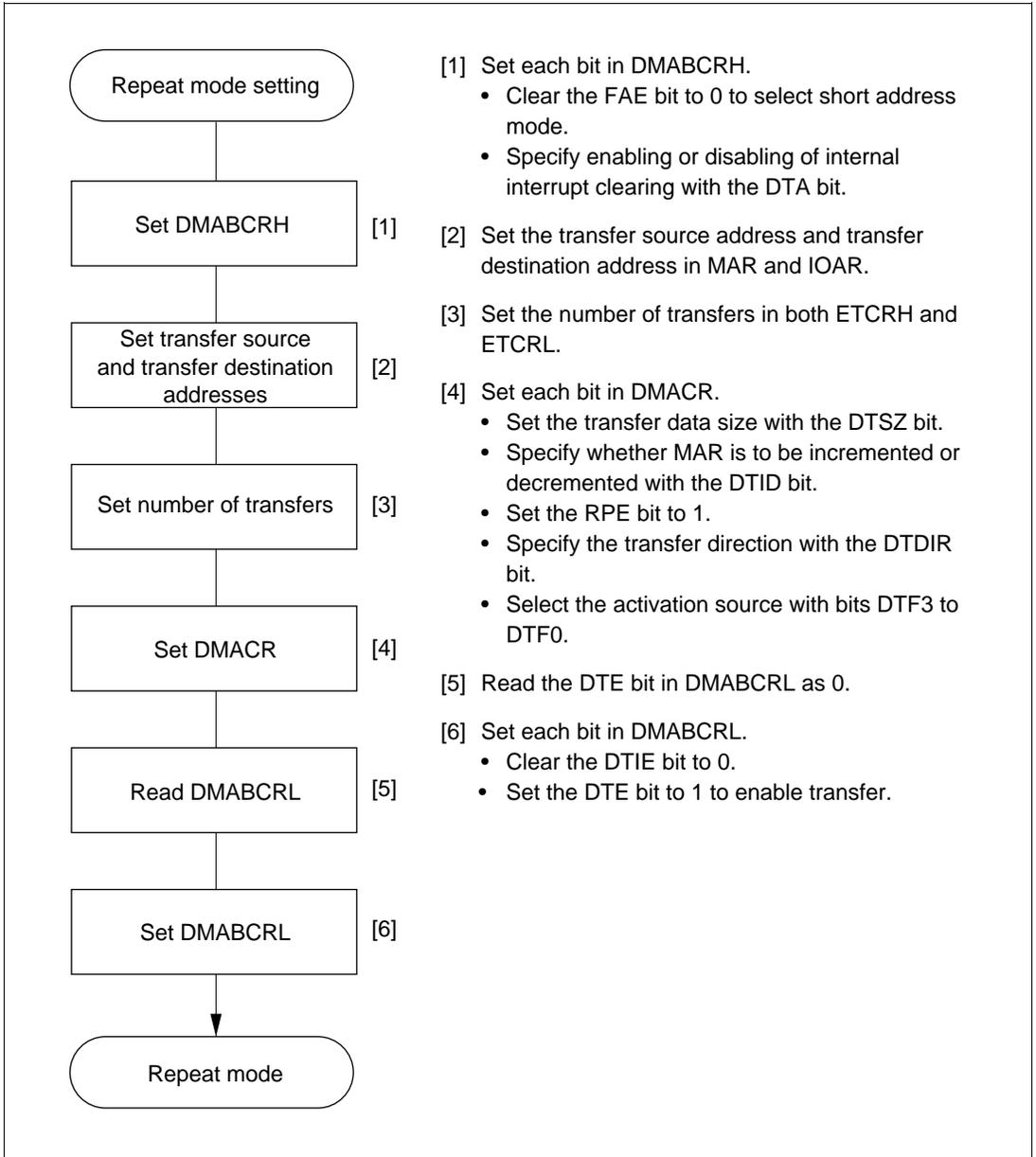
**Figure 7-8 Example of Repeat Mode Setting Procedure**
