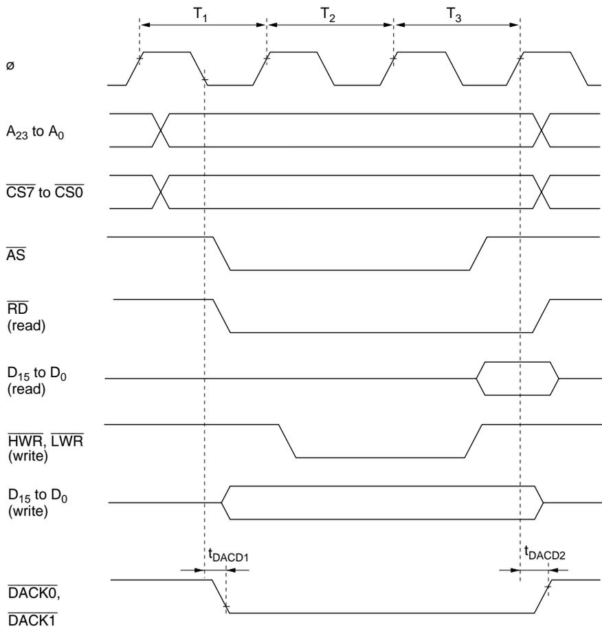
**Figure 22-19 DMAC Single Address Transfer Timing (Three-State Access)**
