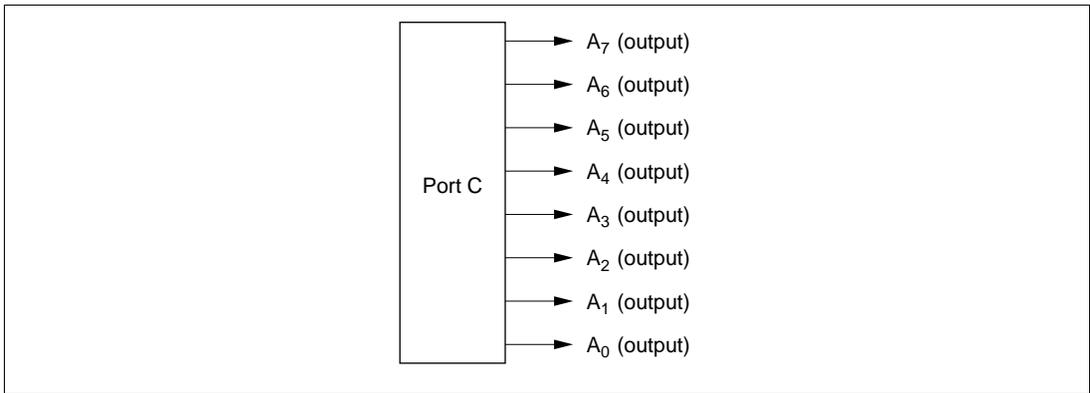
**Figure 9-16 Port C Pin Functions (Modes 4 and 5)**
