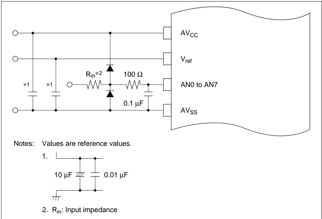
**Figure 16-7 Example of Analog Input Protection Circuit**
