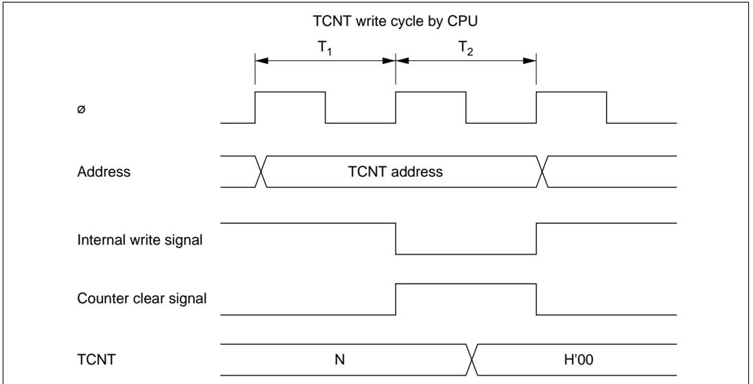
**Figure 12-10 Contention between TCNT Write and Clear**
