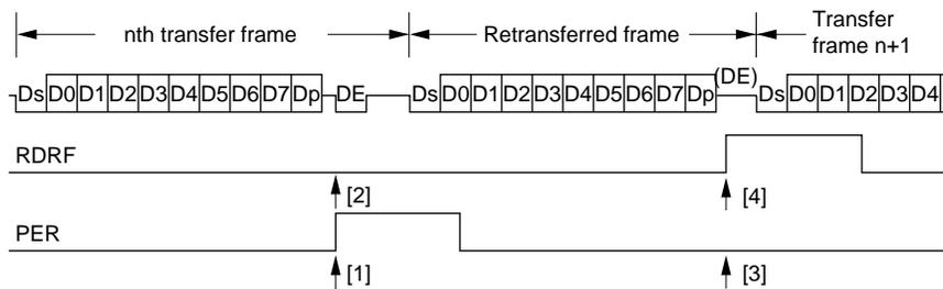
**Figure 15-11 Retransfer Operation in SCI Receive Mode**
