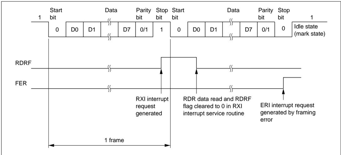
**Figure 14-8 Example of SCI Operation in Reception
