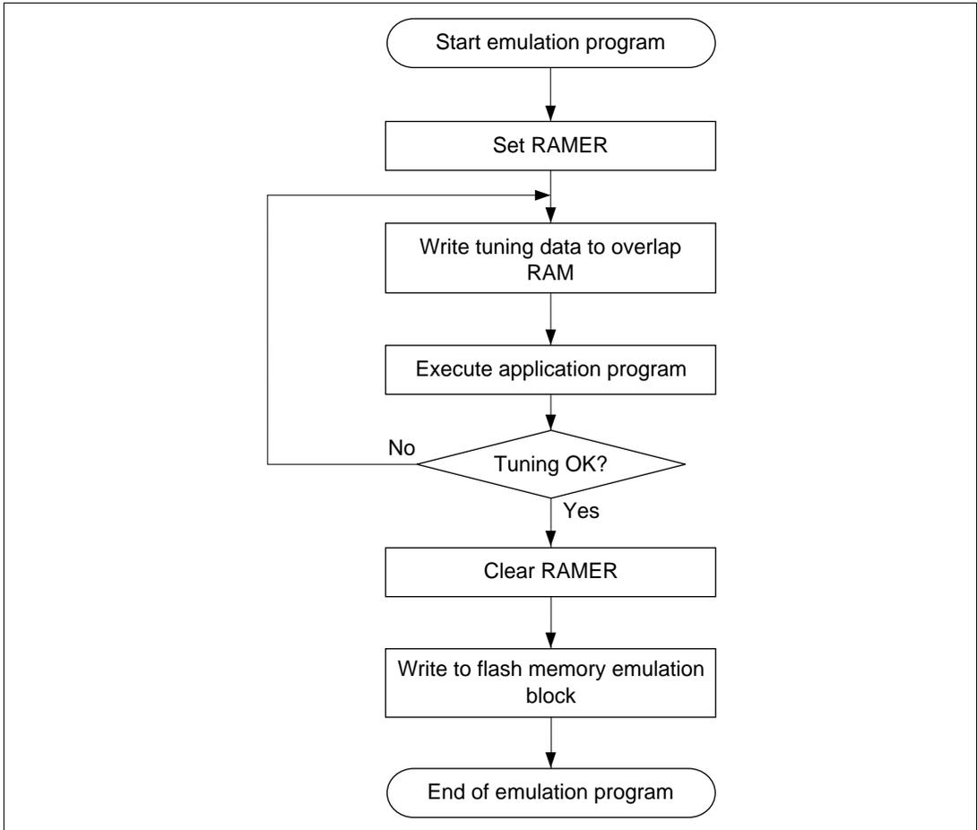
Figure 19-22 Flowchart for Flash Memory Emulation in RAM
