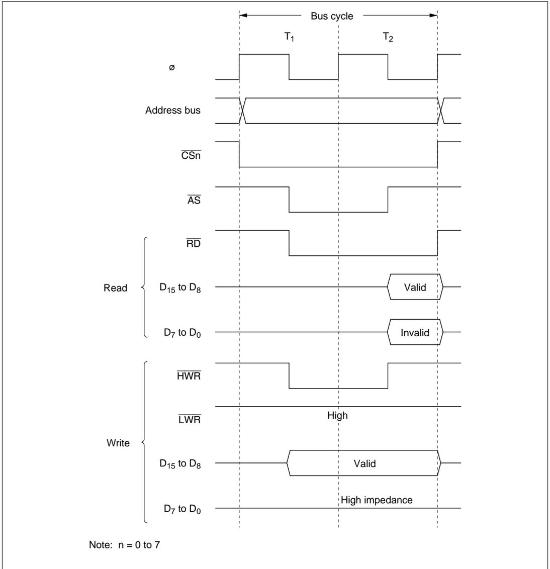
Figure 6-6 Bus Timing for 8-Bit 2-State Access Space
