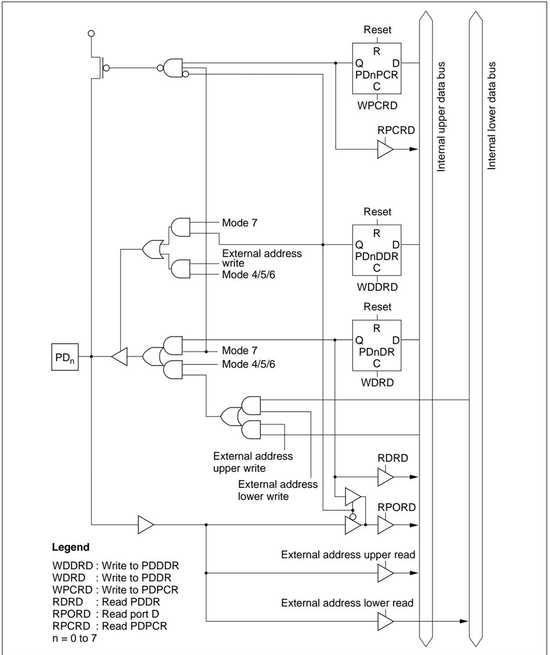
Figure C-10 Port D Block Diagram (Pin  $PD_n$ )
