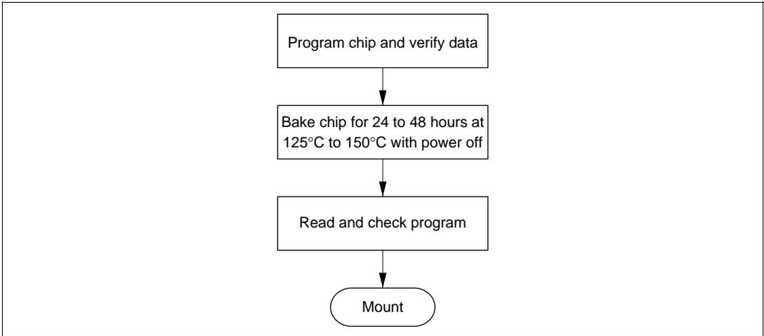
**Figure 19-6 Recommended Screening Procedure**
