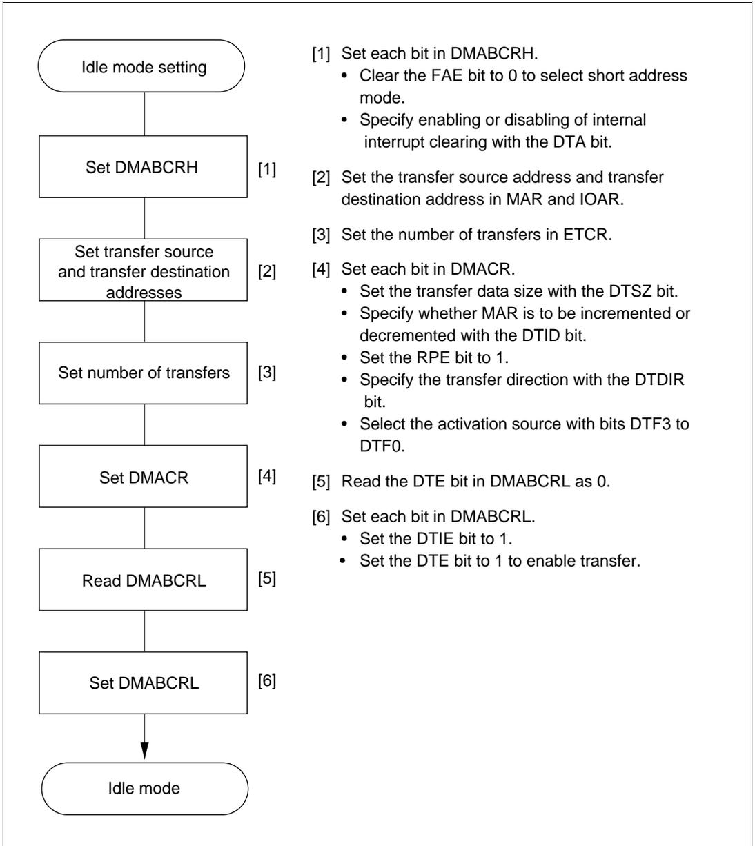
**Figure 7-6 Example of Idle Mode Setting Procedure**
