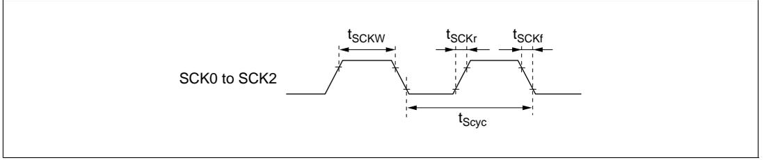
**Figure 22-30 SCK Clock Input Timing**
