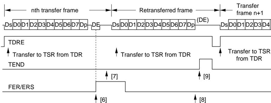
**Figure 15-12 Retransfer Operation in SCI Transmit Mode**
