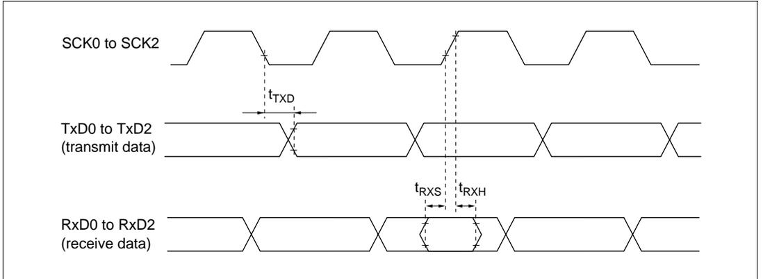
**Figure 22-31 SCI Input/Output Timing (Clock Synchronous Mode)**
