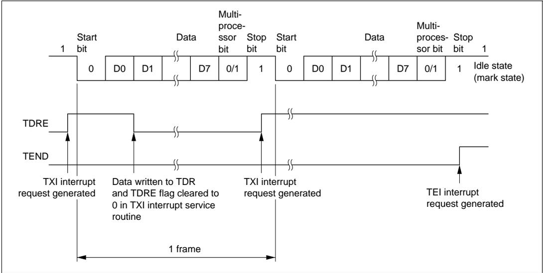
**Figure 14-11 Example of SCI Operation in Transmission
