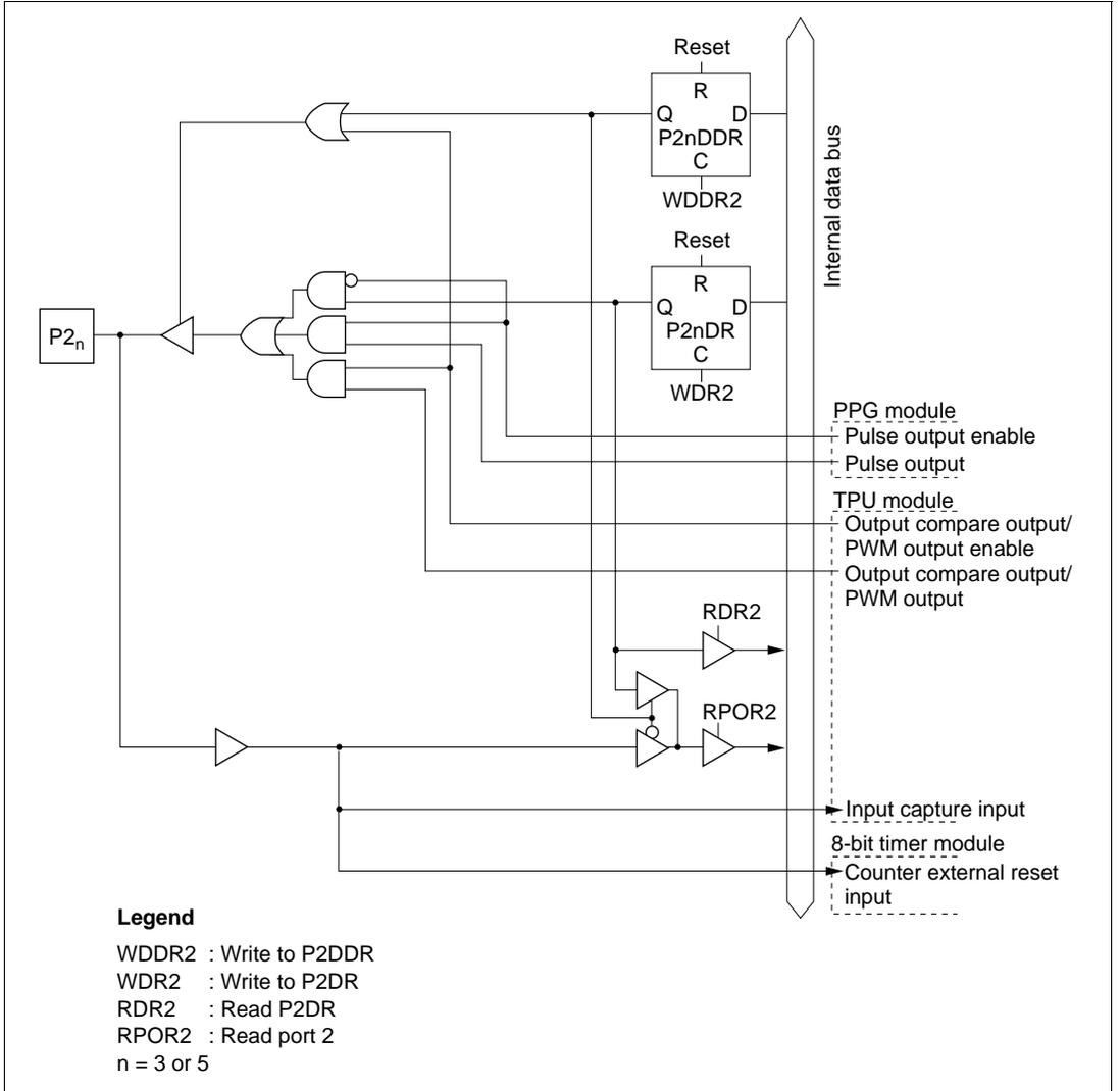
Figure C-2 (c) Port 2 Block Diagram (Pins P2<sub>3</sub> and P2<sub>5</sub>)
