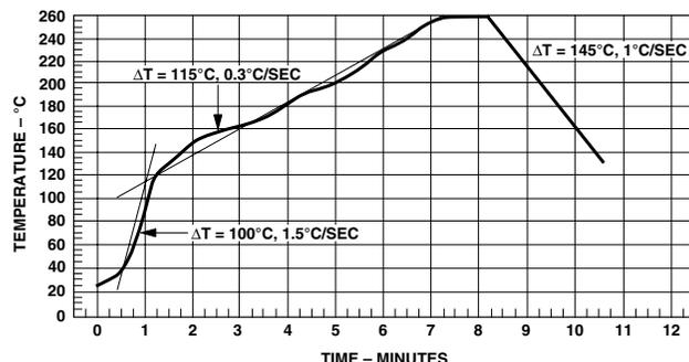
(NOTE: USE OF NON-CHLORINE ACTIVATED FLUXES IS RECOMMENDED.)
