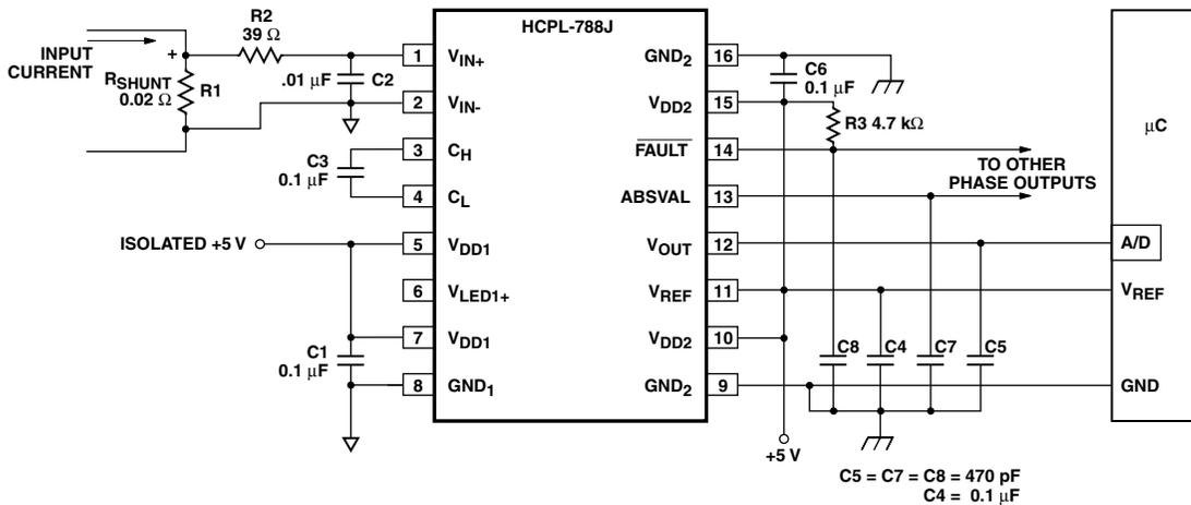
Figure 25. Recommended Applications Circuit.
