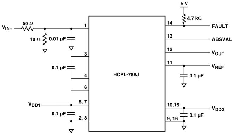
Figure 20. AC Test Circuit.
