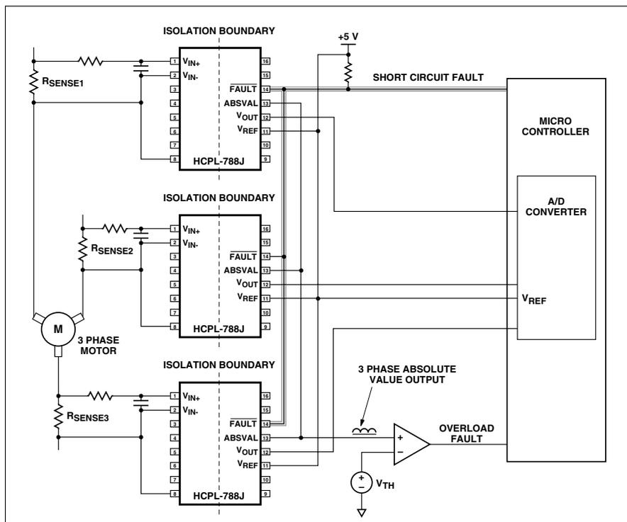
Agilent Technologies Isolation Amplifier with Short Circuit and Overload Detection makes **motor phase current sensing compact, affordable and easy-to-implement** while satisfying worldwide safety and regulatory requirements.
