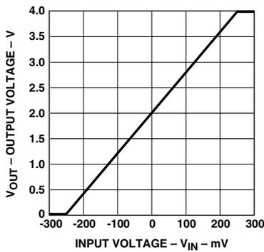
Figure 6.  $V_{OUT}$  vs.  $V_{IN}$ .
