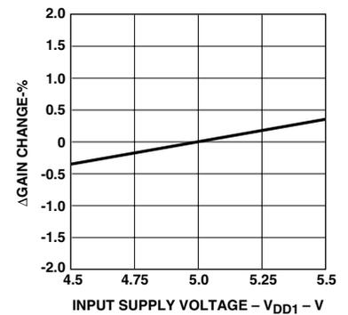
Figure 8. Gain Change vs.  $V_{DD1}$ .
