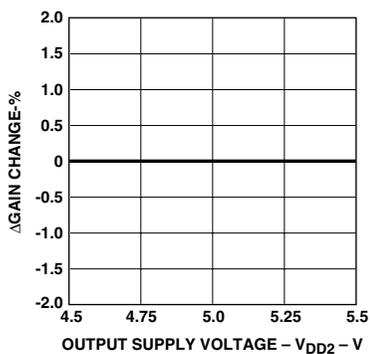
Figure 9. Gain Change vs.  $V_{DD2}$ .
