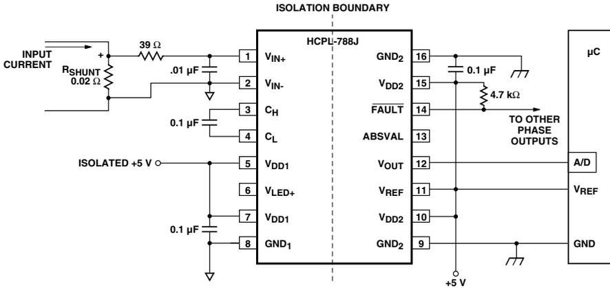
**Figure 1. Current Sensing Circuit.**
