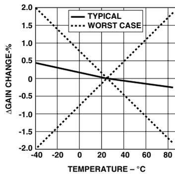
Figure 7. Gain Change vs. Temperature.
