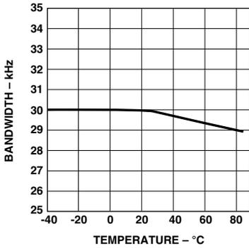
**Figure 12. Bandwidth vs. Temperature.**
