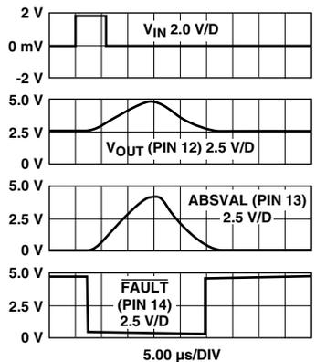
**Figure 18. Detection of 6  $\mu s$  Fault 0 to 2 V to 0 Input, at  $V_{REF} = 5 V$ .**
