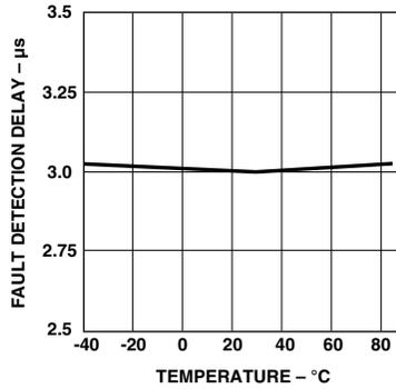
**Figure 13. FAULT Detection Delay vs. Temperature.**
