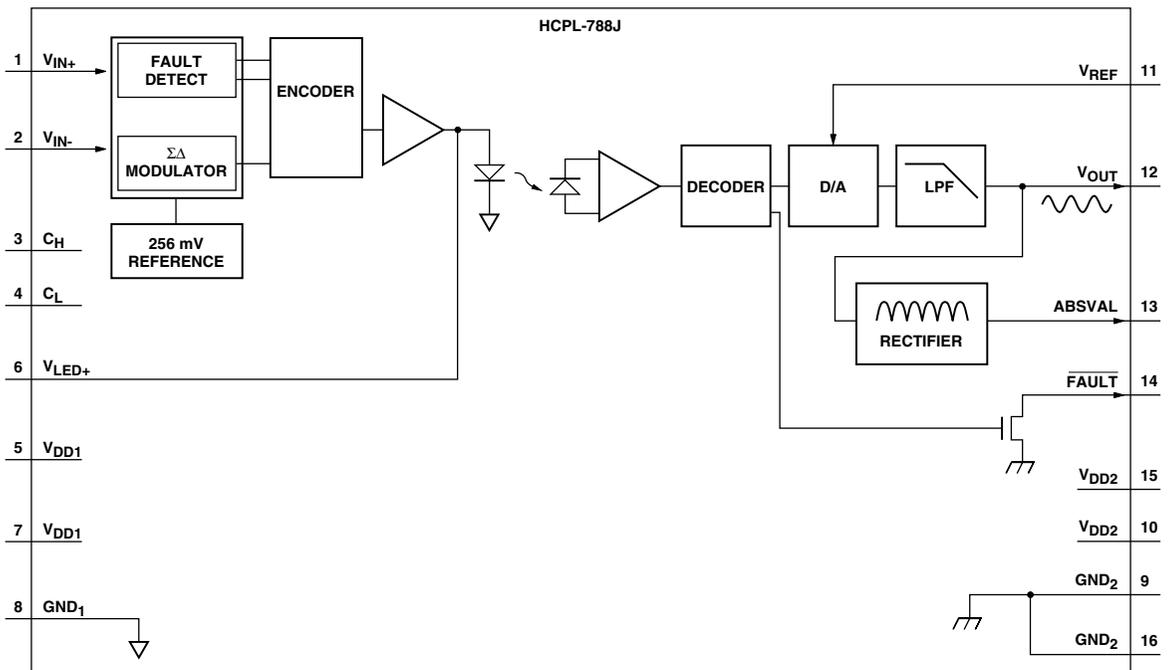
Figure 21. Internal Block Diagram.
