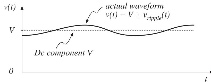
In a well-designed converter, the output voltage ripple is small. Hence, the waveforms can be easily determined by ignoring the ripple:
