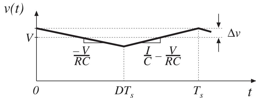
Change in capacitor voltage during subinterval 1 is (*slope*) (*length of subinterval*):
