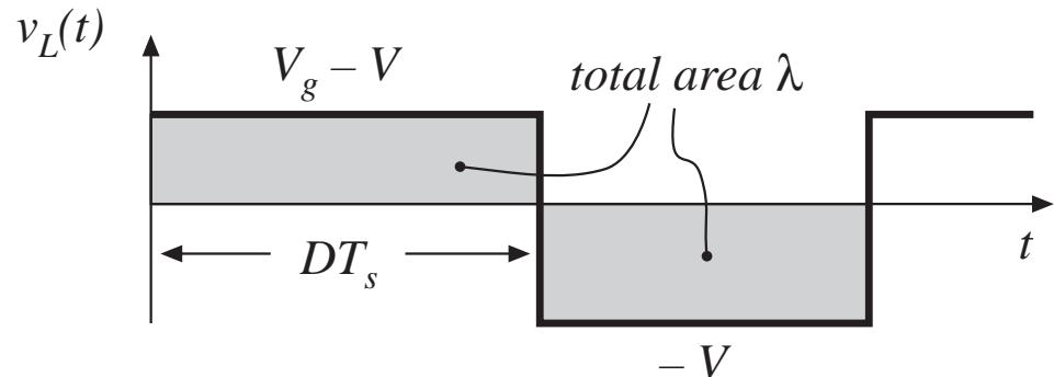
Integral of voltage waveform is area of rectangles:
