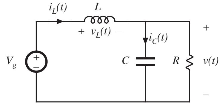
*Knowing the inductor voltage, we can now find the inductor current via*
